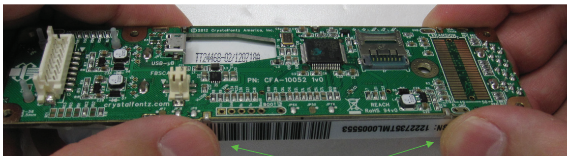
Figure 21. Handling Caution To Avoid Damaging Flat Flex Cable
