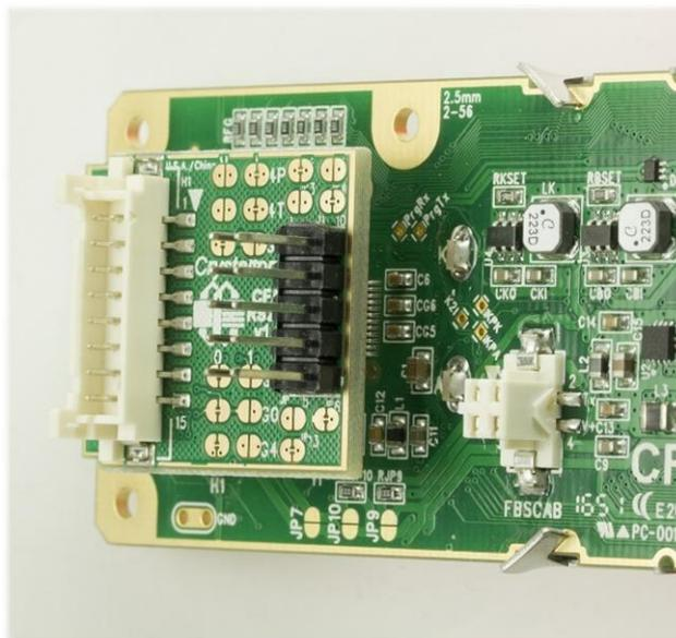
Figure 2. Angled View of CFA-RS232 Level Translator Mounted on CFA Module
