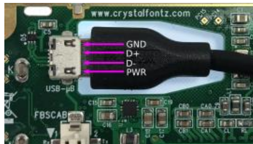
Figure 9. Connecting 5v Power Through USB
