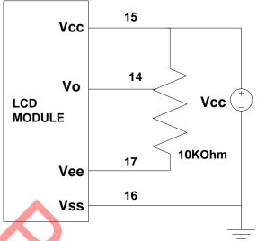
Contrast adjust by using internal Negative (Positive) voltage generator
