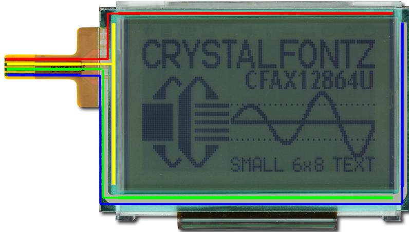
Figure 2. Touch Screen Pinout Details
