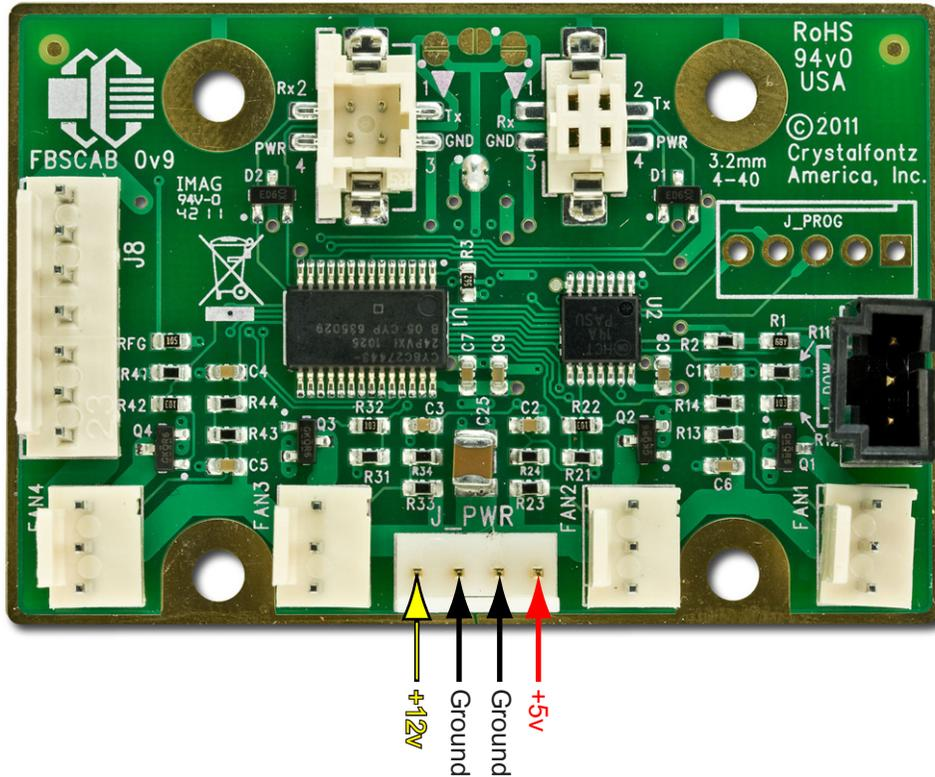
Figure 4. Location of Power Connection (J\_PWR)
