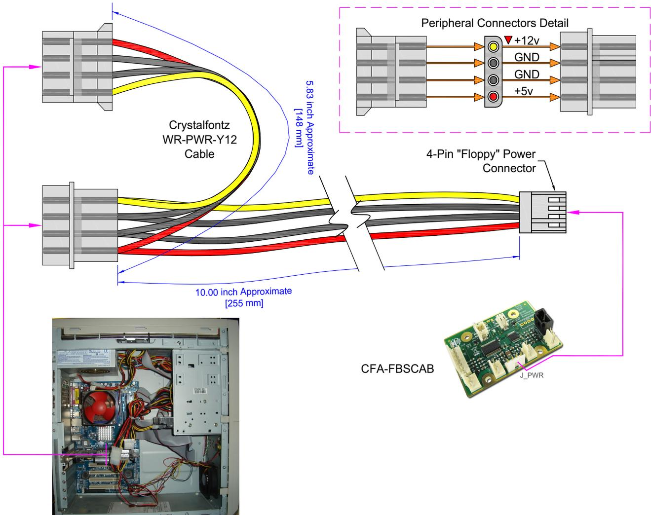
Figure 5. CrystalFontz WR-PWR-Y12 Power Cable
