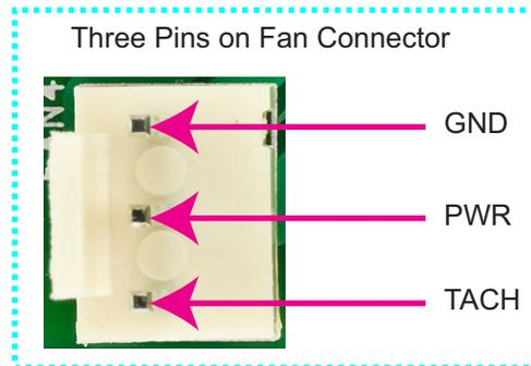
Figure 6. Location of Fan Connectors (FAN1 to FAN4)
