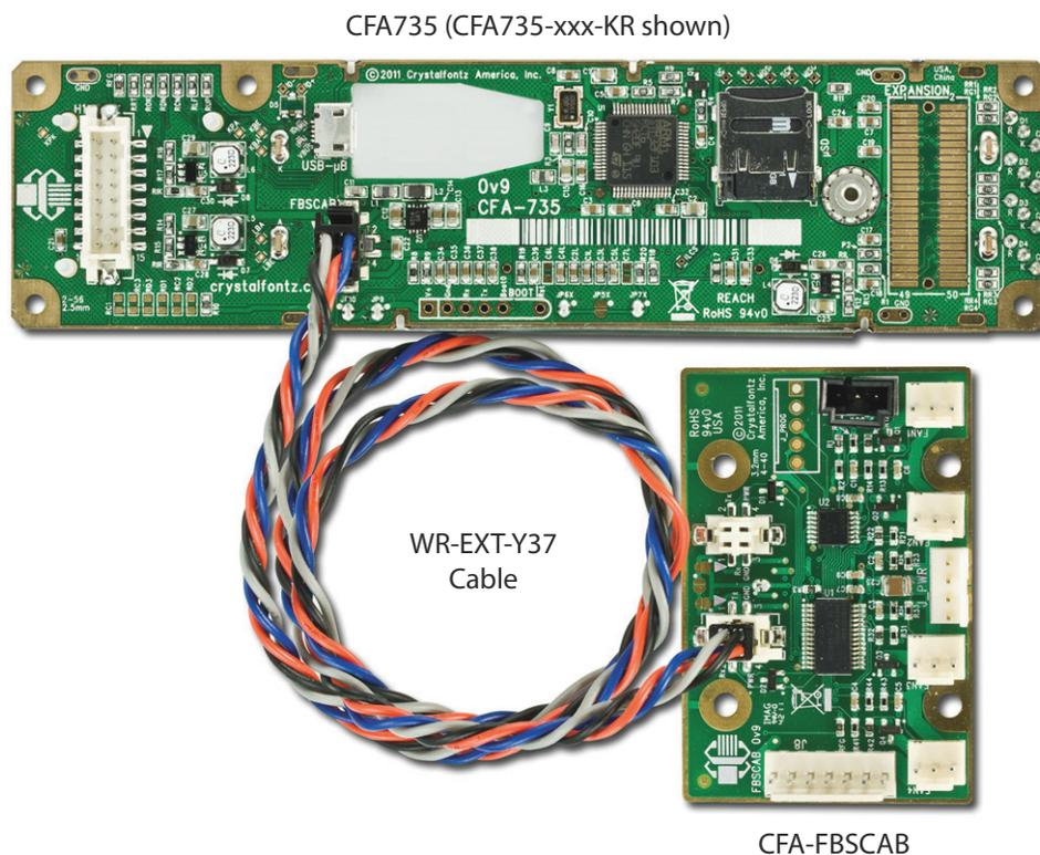
Figure 3. CFA735 Connected to a CFA-FBSCAB Using a WR-EXT-Y37 Cable
