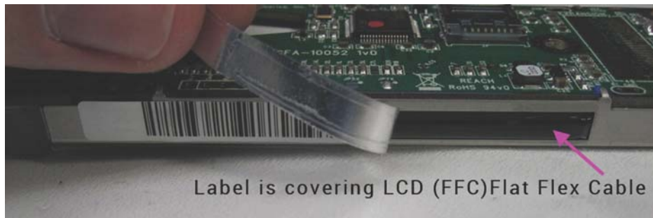
Bent FFC (Flat Flex Cable) is under the label.
