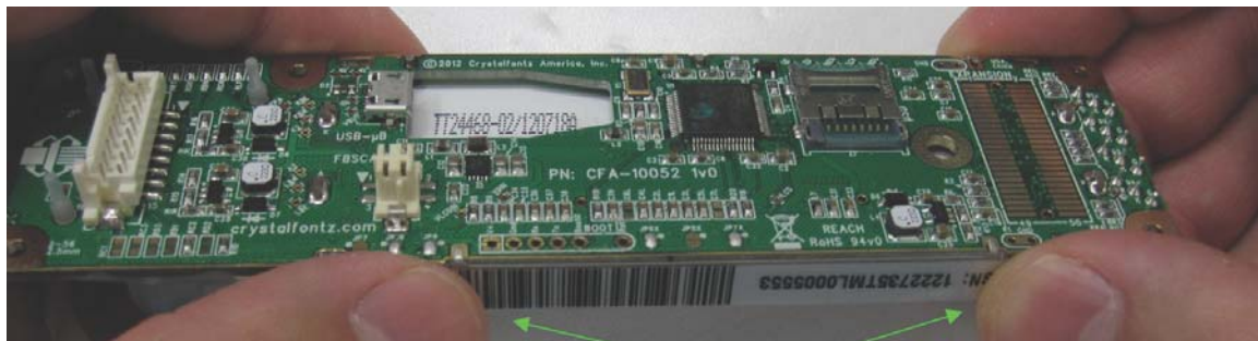
Figure 23. Handling Caution to Avoid Damaging Flat Flex Cable
