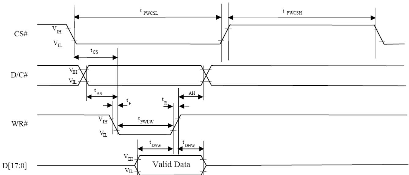
**Figure 7-4: Parallel 8080-series Interface Timing Diagram (Read Cycle)**
