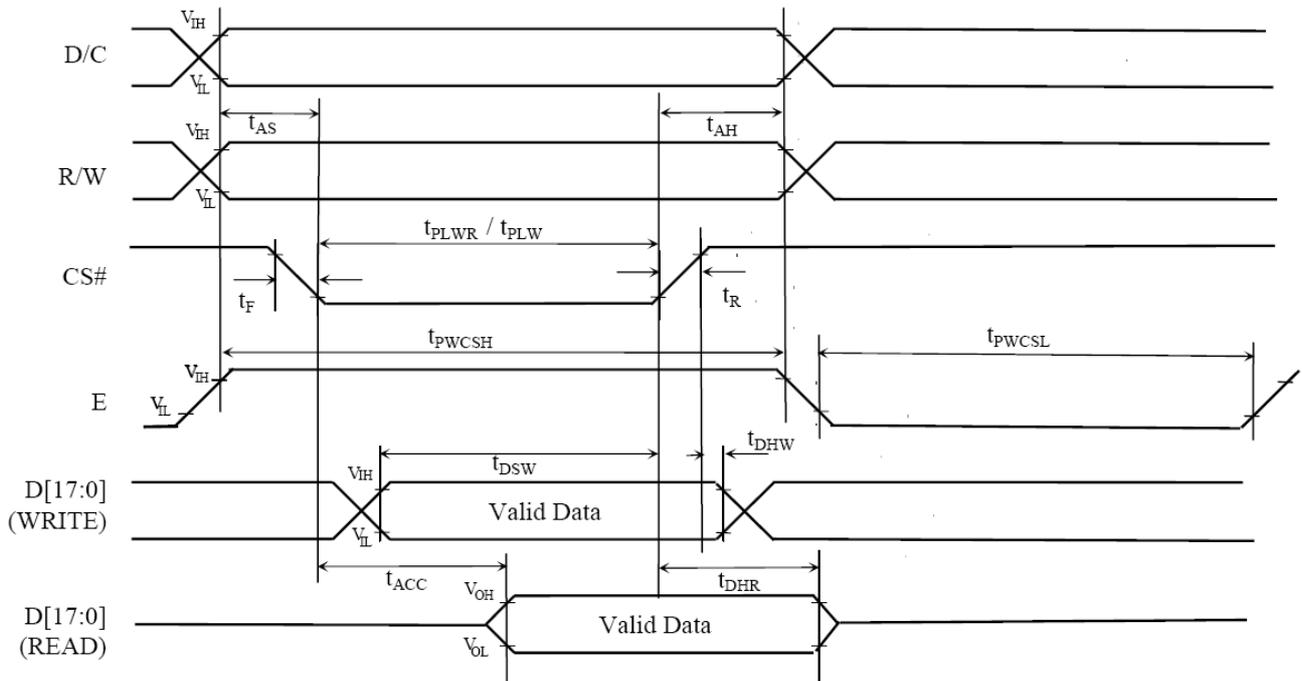
**Table 7-5: Parallel 6800-series Interface Timing Characteristics (Use E as clock)**
