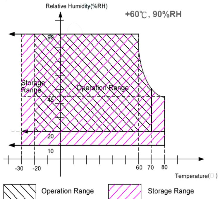
Note 4: In case of temperature below 0°C, the response time of liquid crystal (LC) becomes slower and the color of panel darker than normal one.
