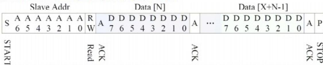
AS FOR STANDARD CTPM, HOST NEED TO USE BOTH INTERRUPT CONTROL SIGNAL AND SERIAL DATA INTERFACE TO GET THE TOUCH DATA, HERE IS THE TIMING TO GET TOUCH DATA.
