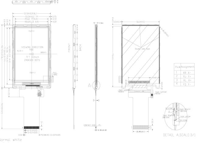
Display type:TFT/Normal white Display mode:Transmissive Viewing direction: 9:00 Driver ID:TM3225C INterface t&pstomer Define Logic volatage: 2.8?&.3 Backlight: White LED(4-LED serial) Vled=12.8±0.5V Iled=20mA Dperating temprature: -20°C ~ +70°C Storage temprature: -30°C ~ +80°C Interfaceonnector: FPC
