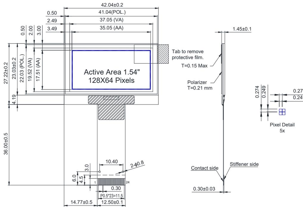
Tolerance  $\pm 0.3\text{mm}$  unless otherwise specified.
