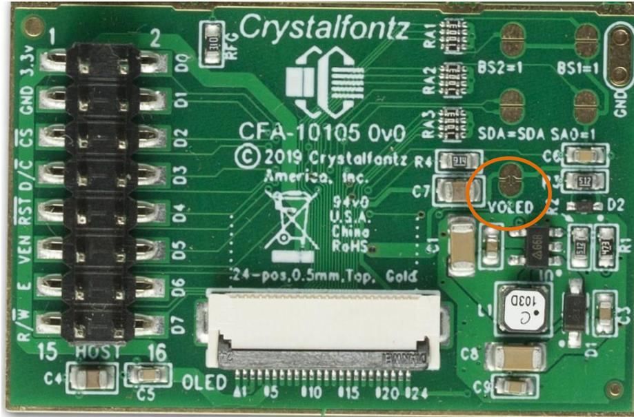
This jumper is shipped closed, tying VOLED high and thus enabled. To manually control VOLED Enable, open this jumper. Once open, Pin 11, VEN, on HOST will control VOLED Enable.
