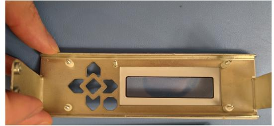
Step 2: Remove screen protector and place display in bracket. Tighten the nuts onto the screws.
