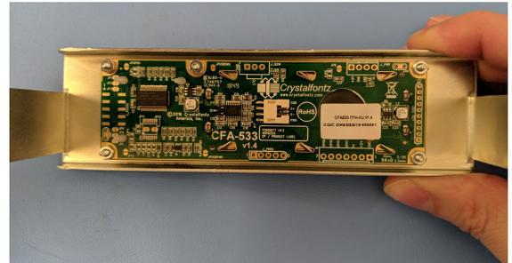
Step 3: Connect a cable between the display and the motherboard. The CFA533 and CFA633 use a special low profile USB cable, available on our website.
