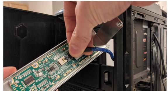
Step 4: Secure the module to the PC case
