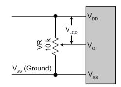
Start with an initial value of  $V_0 = +1v$  ( $V_{LCD} = +4v$ ), and adjust from there.
