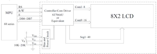
Set  $V_0$  to +1v such that  $V_{LCD}$  = +4v as an initial setting. Using the potentiometer VR, adjust  $V_0$  for optimal display appearance.
