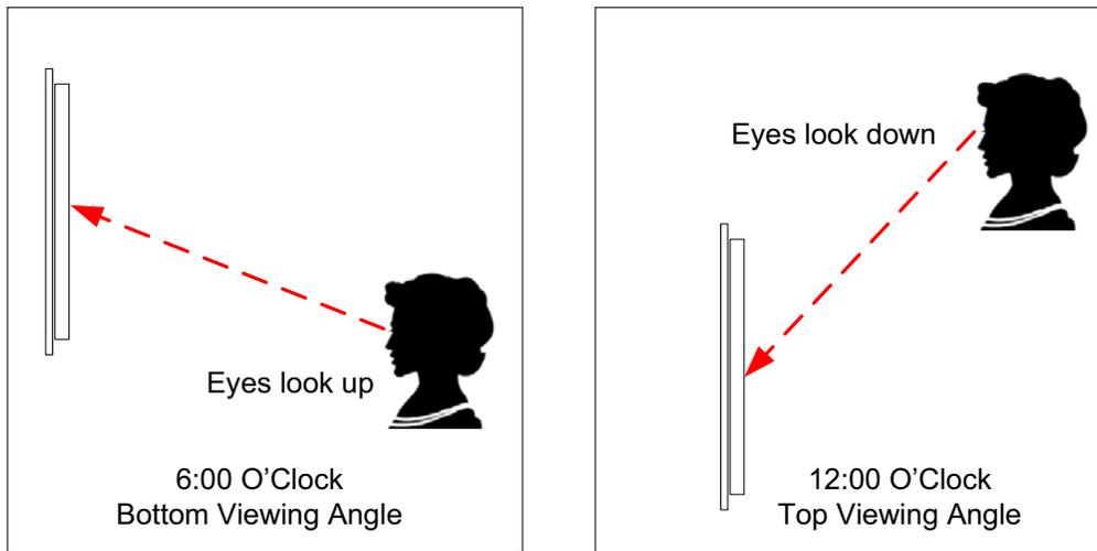
Figure 3. Definition of 6:00 O'clock and 12:00 O'clock Viewing Angles
