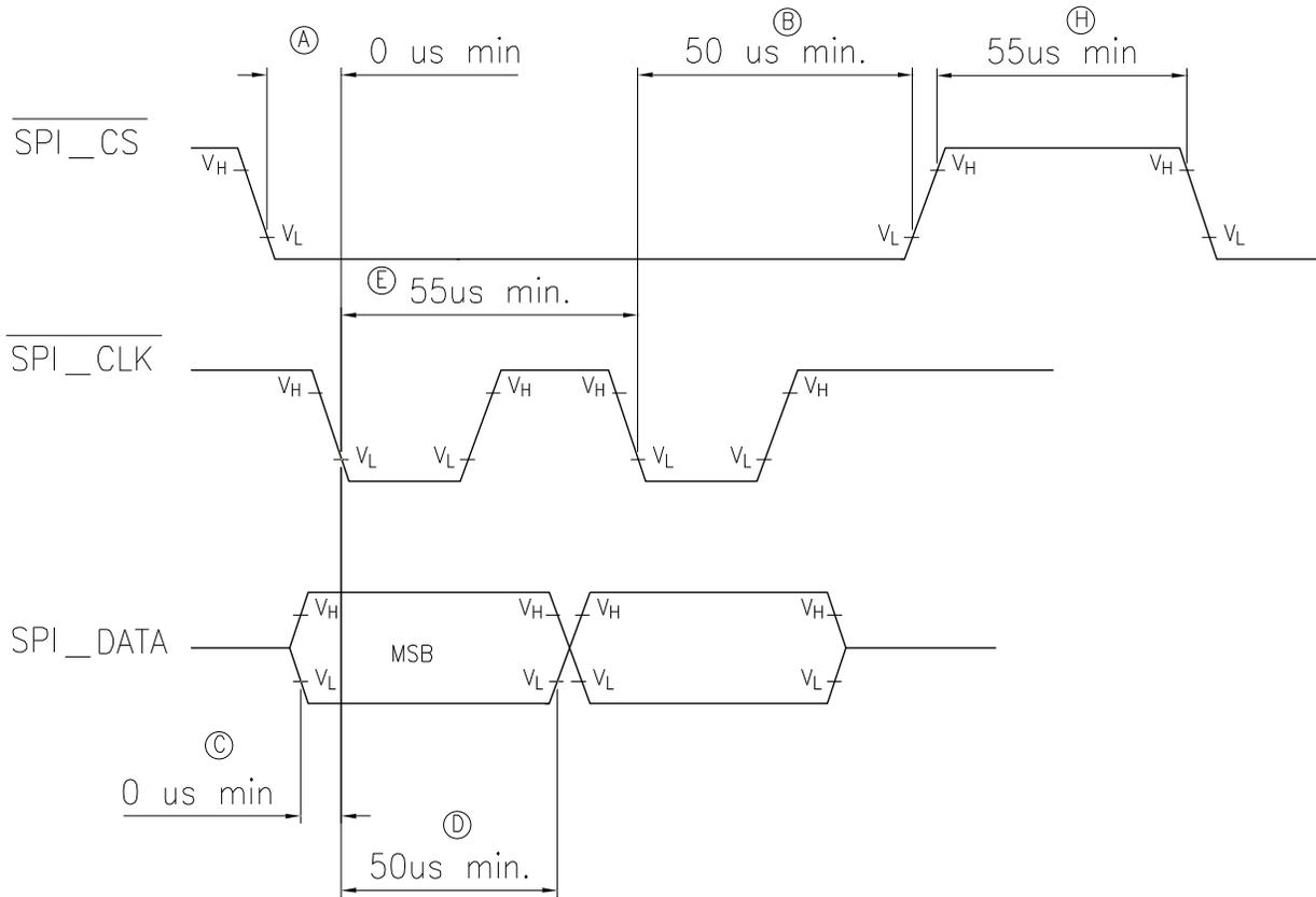
Appendix A Figure 1. CFA634 SPI Timing Diagrams
