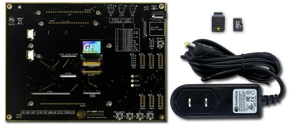
Photo Of Demonstration Board Kit For CFAL9664B-F-B1 OLED Module
