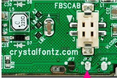
JP10 on the CFA735-xxx-KR is closed by factory default. If you are going to use USB interface while supplying power through H1, you must **open JP10** to prevent back-powering the USB.
