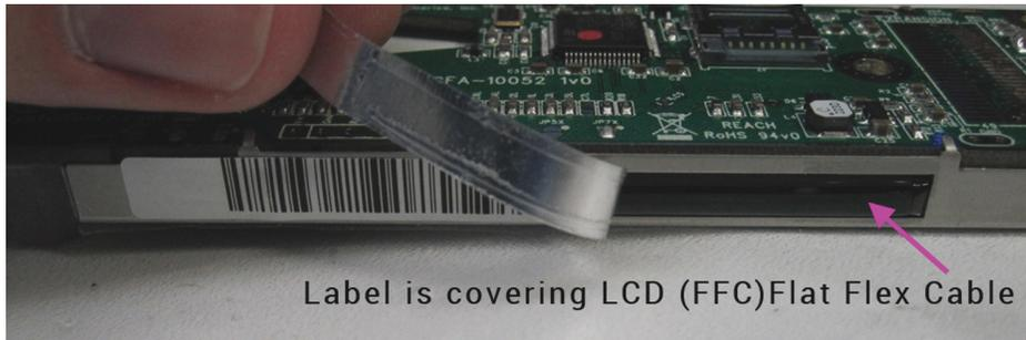
Label is covering LCD (FFC) Flat Flex Cable
