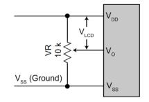
Although a potentiometer is shown as a typical connection,  $V_{\rm O}$  can be driven by a microcontroller, using either a DAC or a filtered PWM. Displays that require  $V_{\rm O}$  to be negative may require a level shifting circuit.
