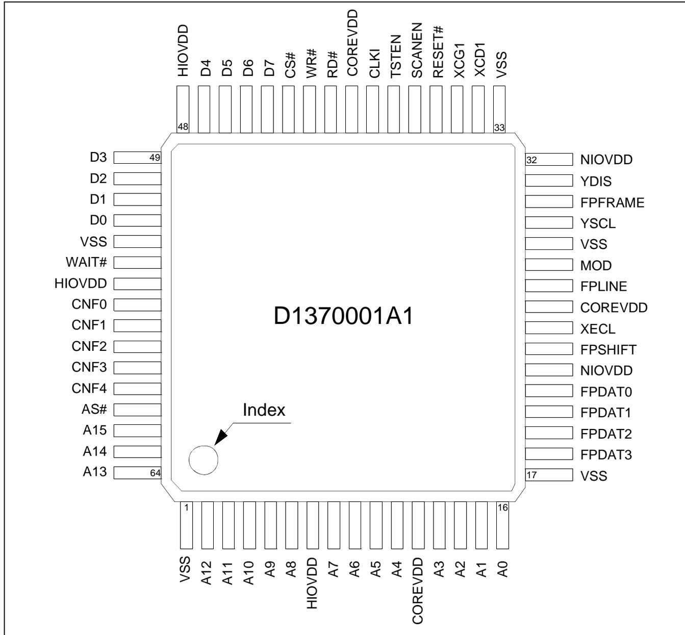
Figure 5-1 Pinout Diagram (TQFP13 - 64 pin)
