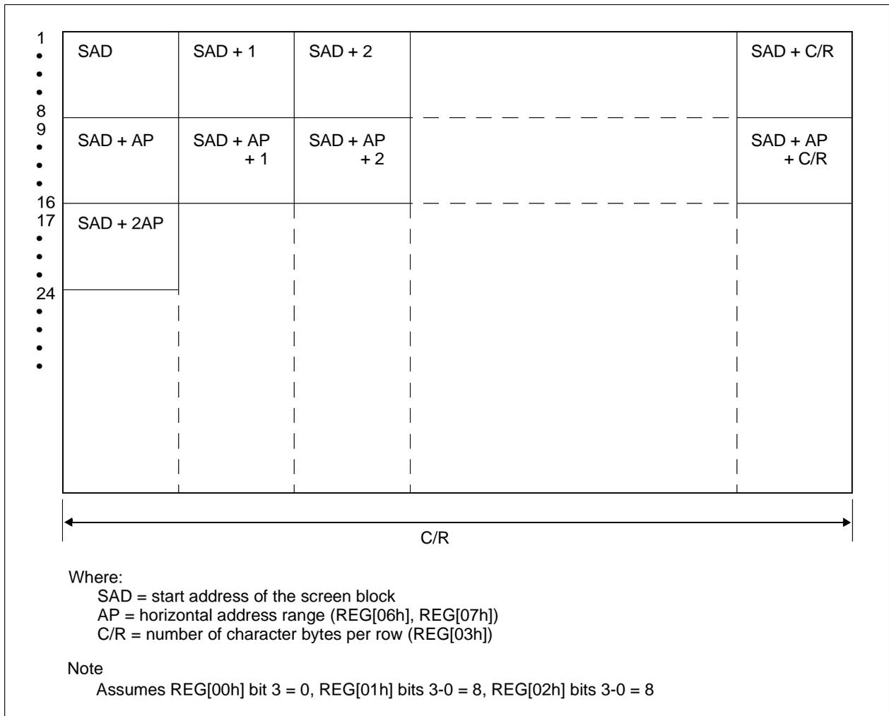
Figure 12-4 Display Addressing in Text Mode Example
