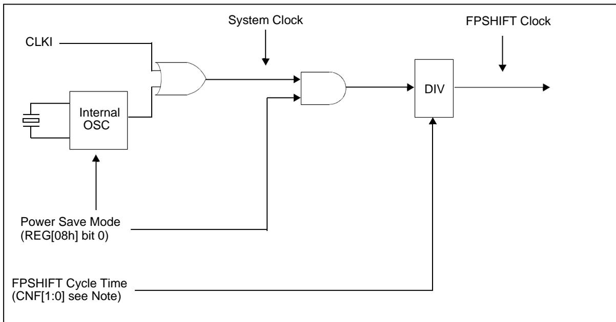
Figure 9-1: Clock Diagram
