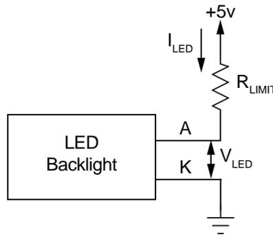
Figure 9. Typical LED Backlight Connections for “Always On”
