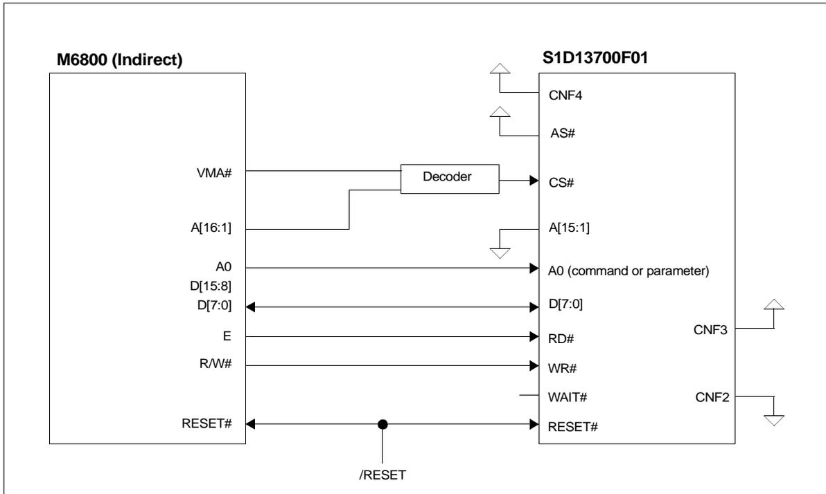
Figure 3-5 Indirect M6800 to S1D13700F01 Interface Example
