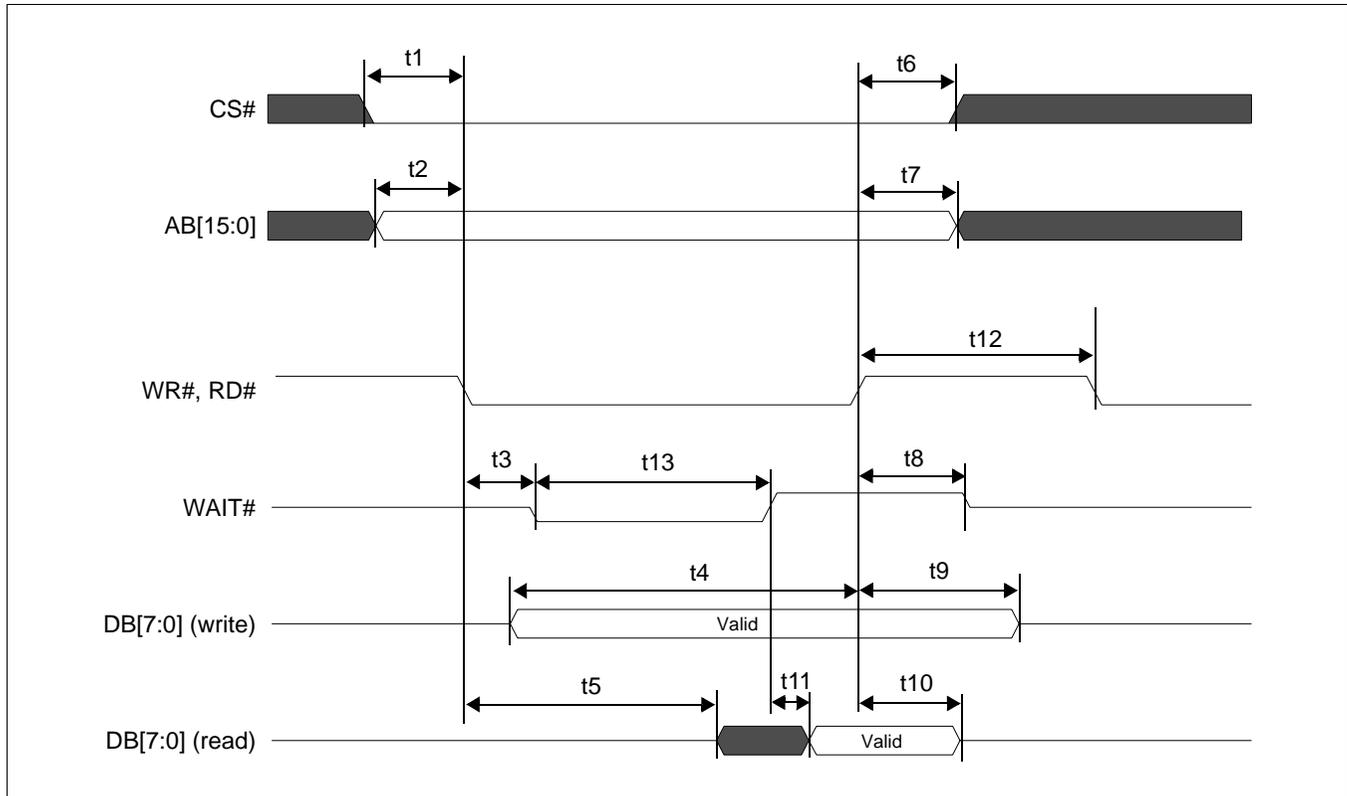
Figure 7-3 Generic Bus Direct/Indirect Interface with WAIT# Timing
