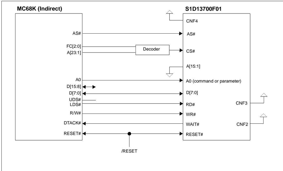
Figure 3-3 Indirect MC68K to S1D13700F01 Interface Example
