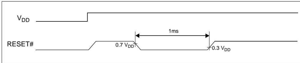
Figure 7-2 Reset Timing
