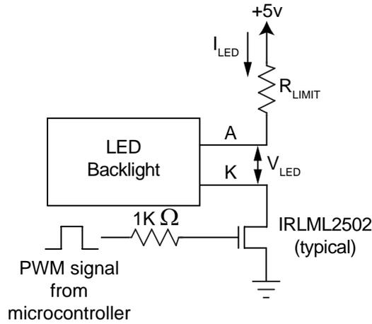
Figure 10. Typical LED Backlight Connections for PWM Dimming
