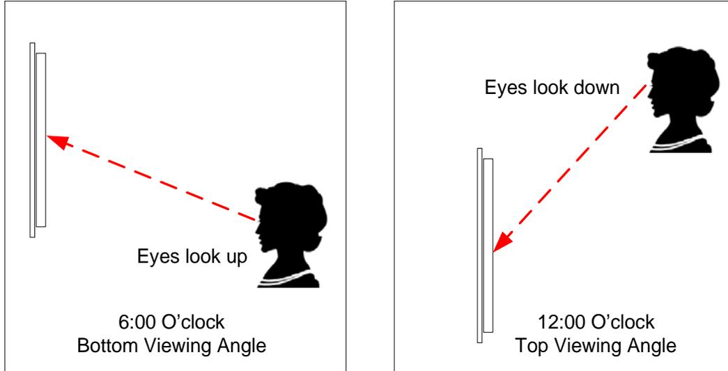
Figure 8. Definition of 6:00 O'Clock and 12:00 O'Clock Viewing Angles
