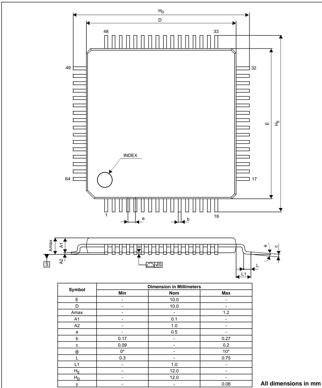
Figure 18-1 Mechanical Drawing TQFP13 - 64 pin
