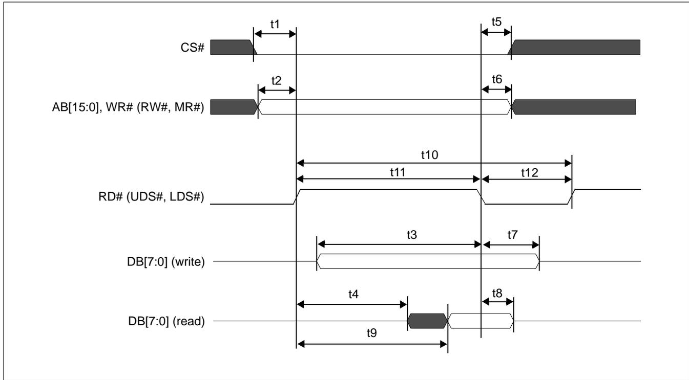
Figure 7-7 M6800 Family Bus Indirect Interface Timing
