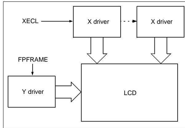
*Figure 10-2 Single Drive Panel Display*
