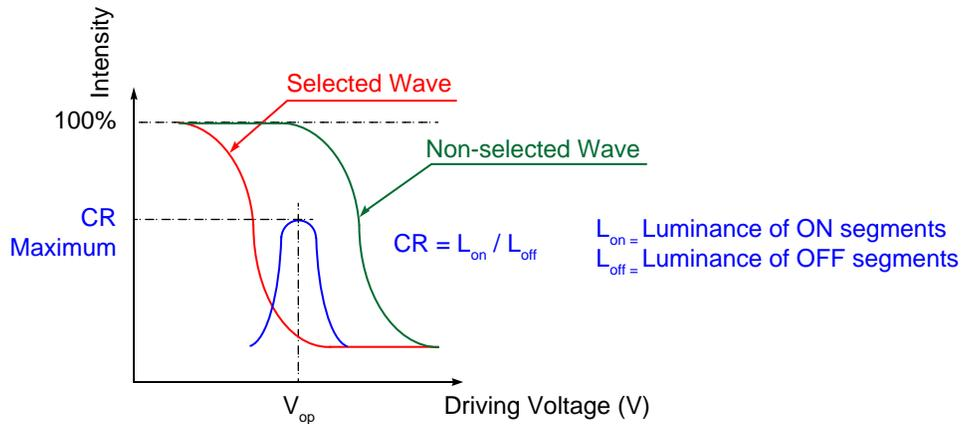
Figure 5. Definition of Operation Voltage ( $V_{OP}$ )
