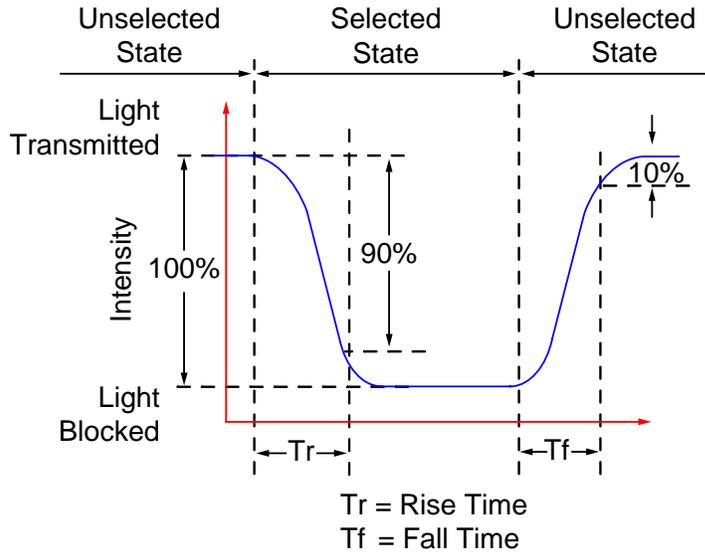
Figure 6. Definition of Response Time ( $T_r$ ,  $T_f$ )
