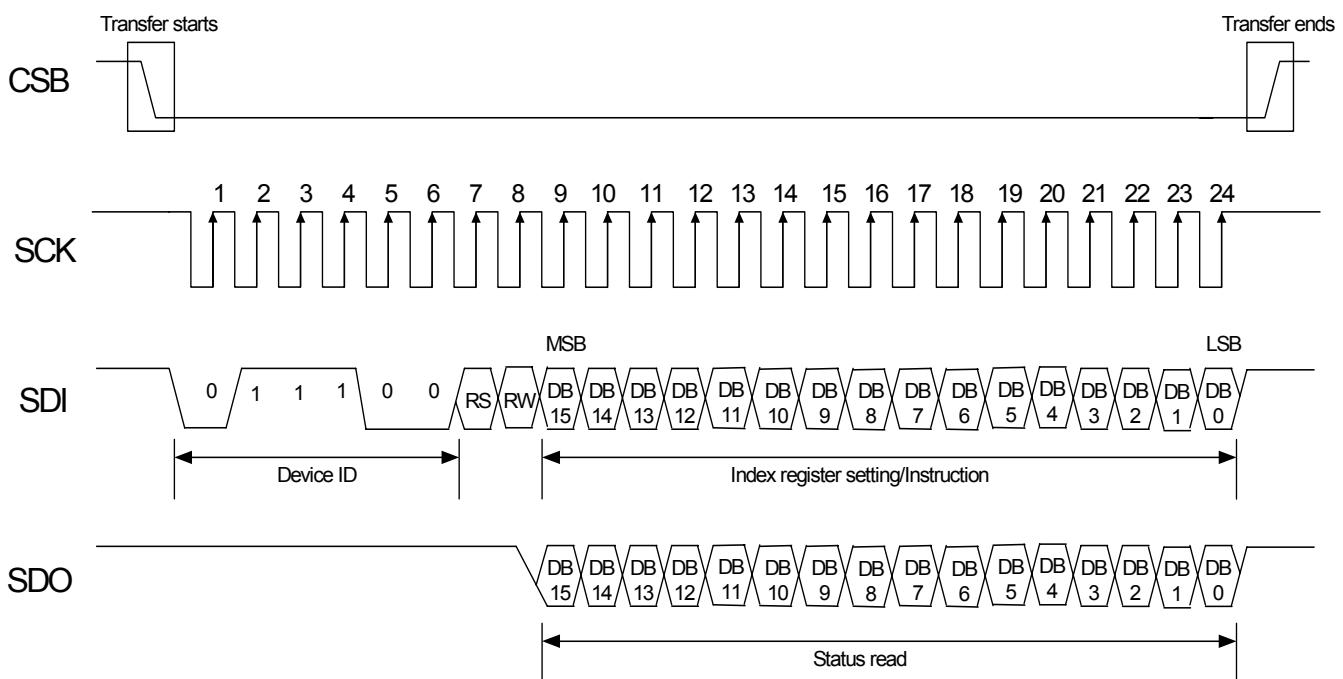
**Figure 6. 1: SPI timing**
