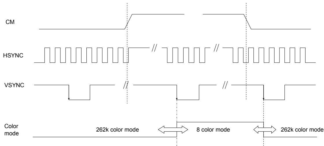
**Note:** The color mode conversion starts at the first falling edge of VSYNC after stage change of CM.
