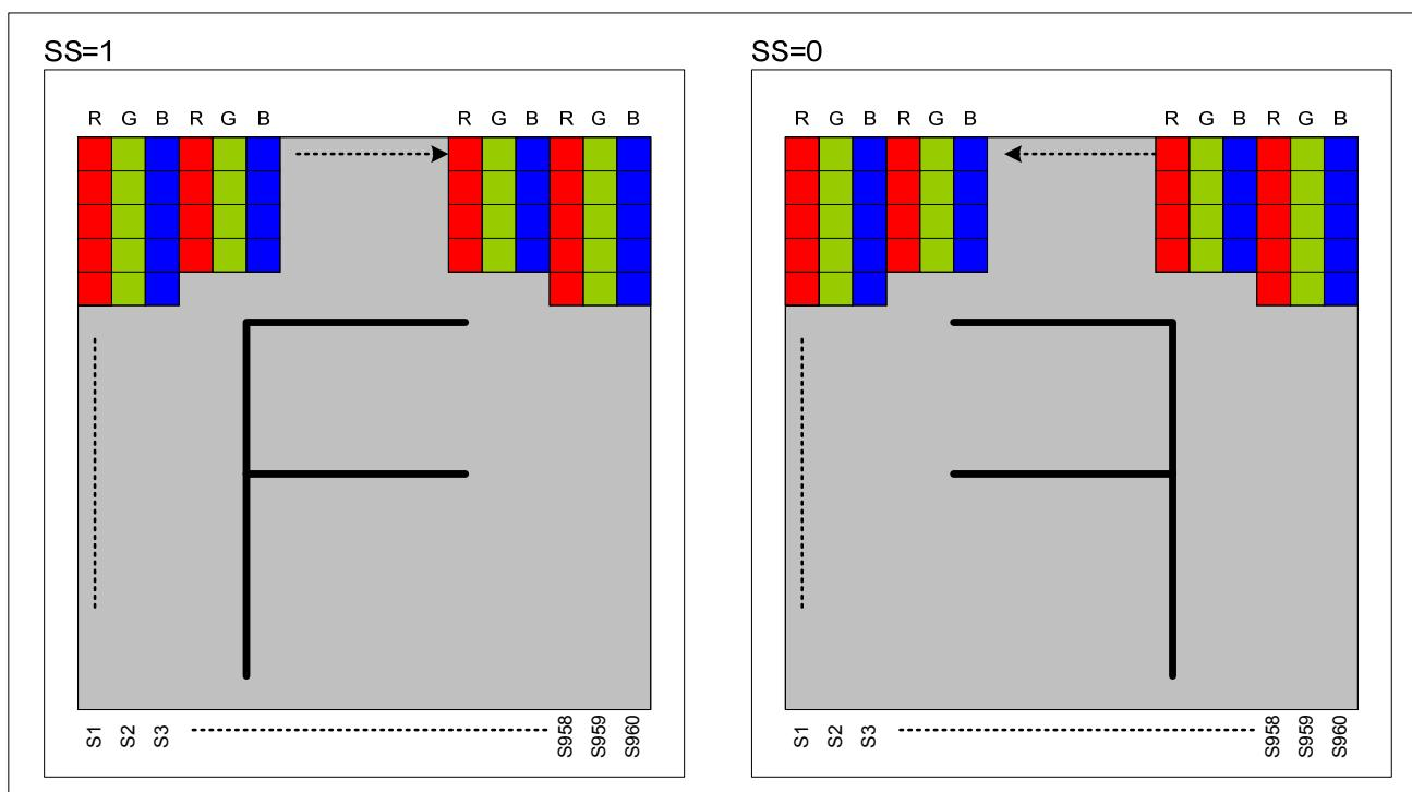
**Figure 7. 26: Display direction according to SS**
