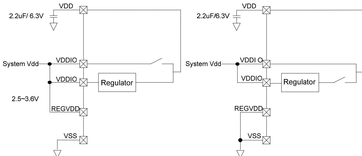
**Figure 14. 2: Power supply pins connections**
