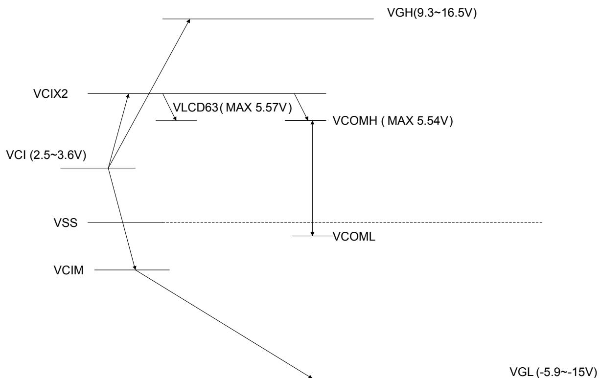
**Note:** The above voltages level assumed 100% efficiency of the internal booster. There has no voltage drop due to resistance from ITO trace of the panel.
