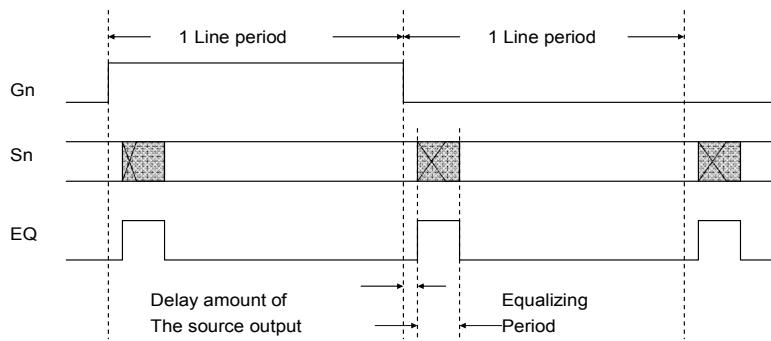
Figure 7.12: EQ timing diagram
