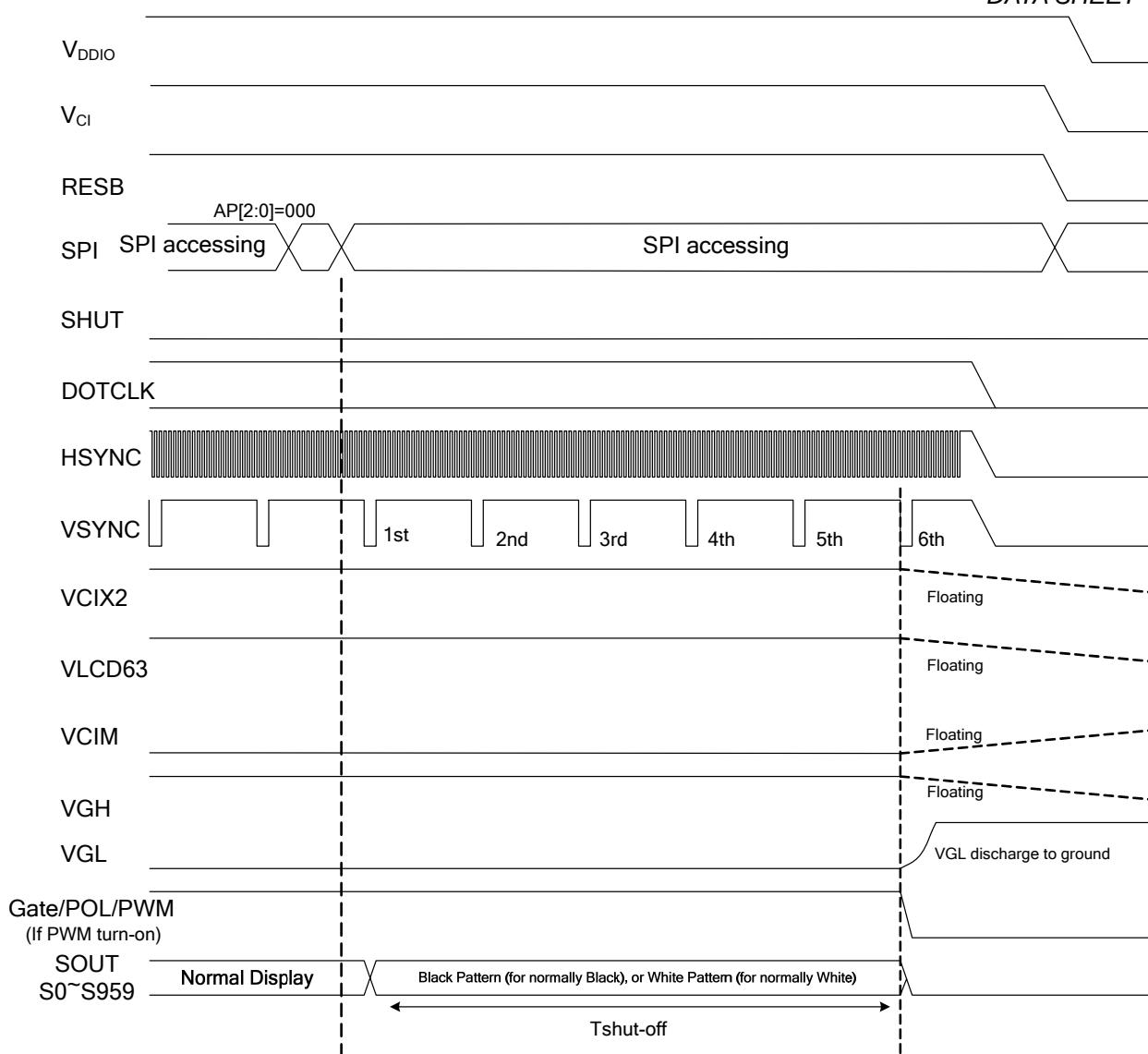
Figure 12. 13: Power down sequence without SHUT
