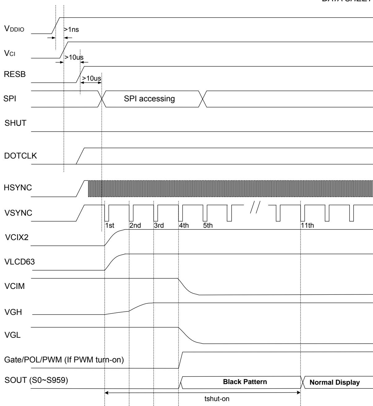
Figure 12. 11: Power up sequence without SHUT
