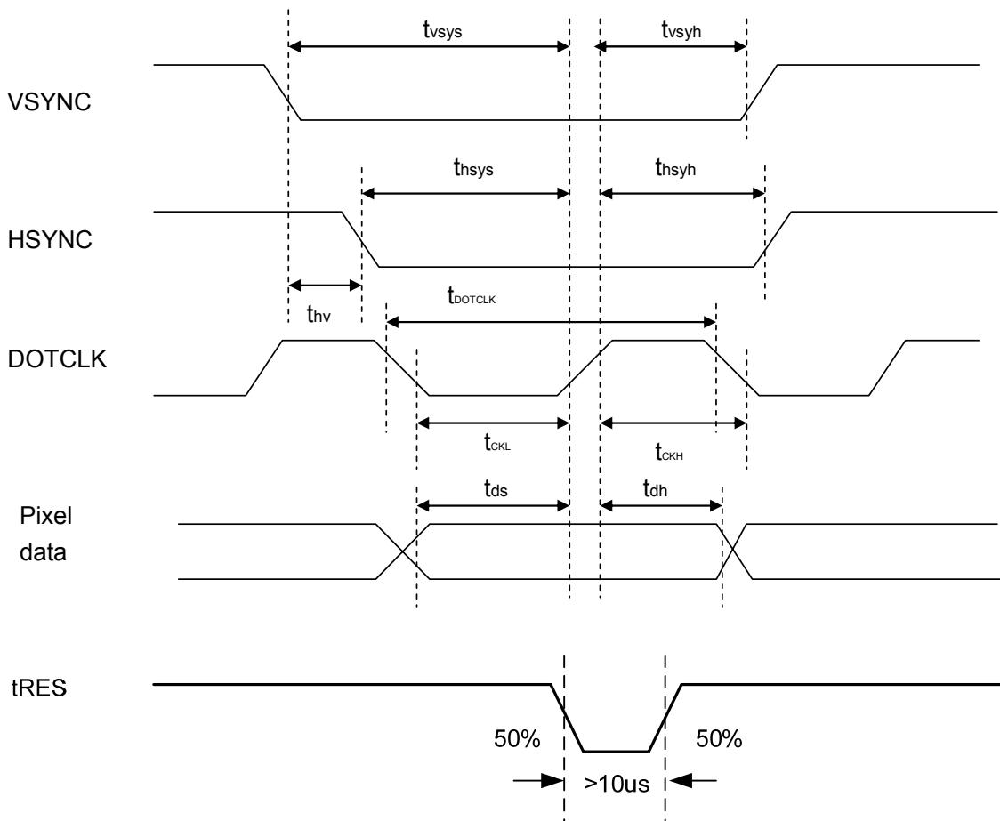
Figure 12. 1: Pixel timing
