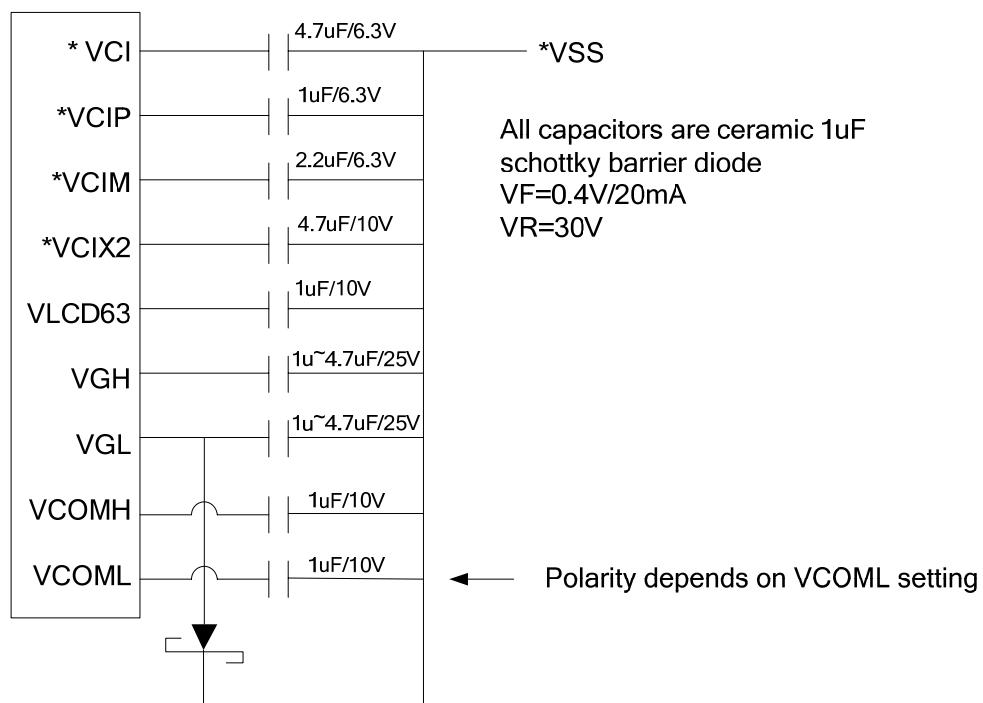
Figure 14. 3: Filtering and charge sharing capacitors
