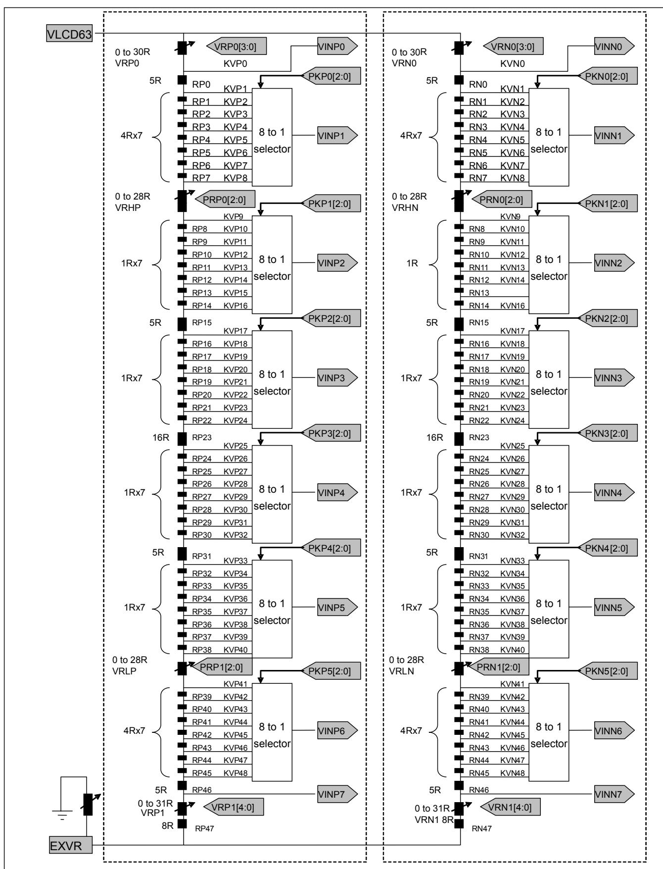
Figure 9.3: Resistor ladder for gamma voltages generation
