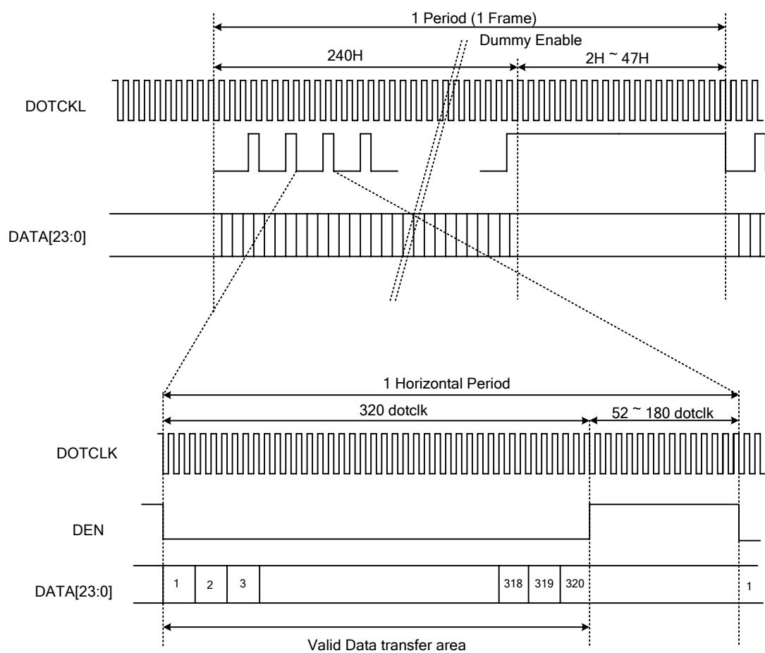
Figure 12.4: Signal timing in DE only mode
