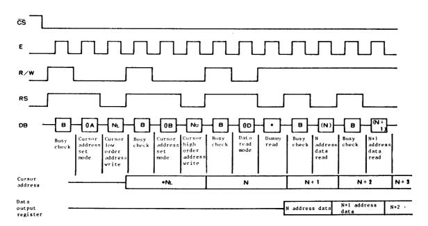
This instruction outputs the contents of data output register on Data Bus (DBO to DB7) and then transfers RAM data specified by a cursor address to the data output register, also increasing the cursor address by 1. After setting the cursor address, correct data is not output at the first read but at the second time. Thus, make one dummy read when reading data after setting the cursor address.
