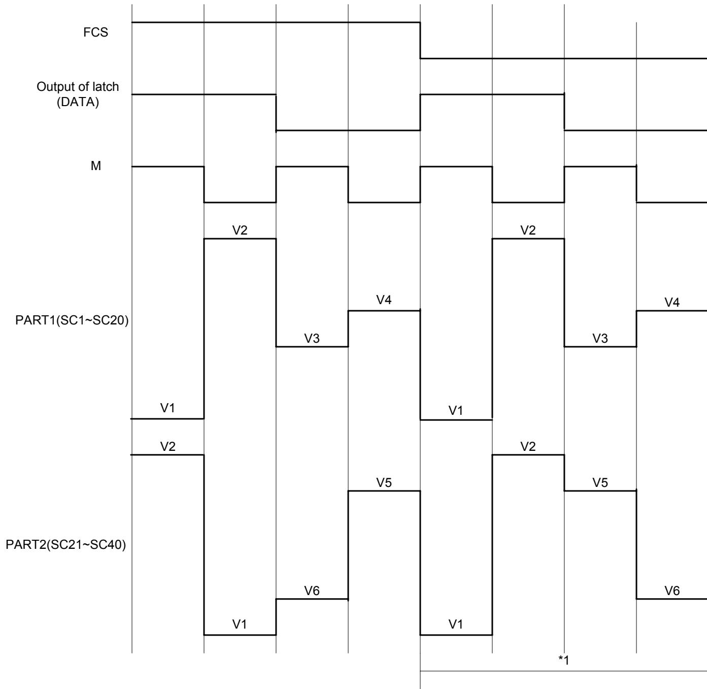
\*1: To use for same function of part1 and part2, V3 and V5, V4 and V6 of power supply for LCD driver are short circuited respectively.
