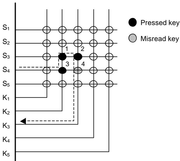
Fig. 1 Miss-recognized key of multi-key scan operation
