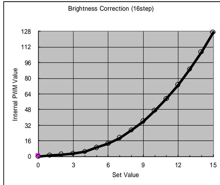
PWM data for Po1~Po4 ports is set as below. First select output port through setting (m) PWM Output Port, and then enable the LED Port mode through setting (n) PWM Program/Port Mode, then setup the PWM data for the selected output port.
