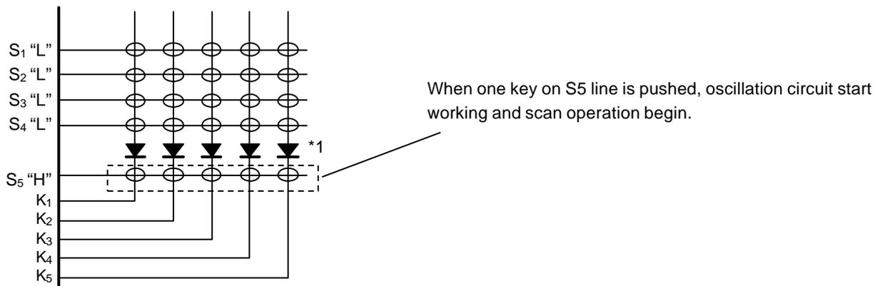
\*1 Under the above Power Save mode, these diodes are used to prevent malfunction during the multi-key scan operation.
