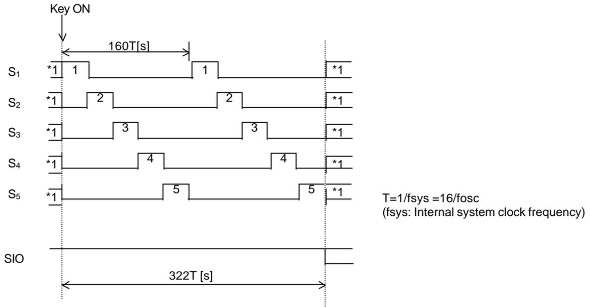
\*1 The state of S1~S5 is decided by (1) PWM Frequency/Po4 (S1) and (n) Power Save Mode. The scan cycle and the timing of key data readout request are the same no matter which Power Save mode is used.
