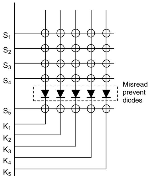
Fig. 3 Connect miss-recognition prevent diodes
