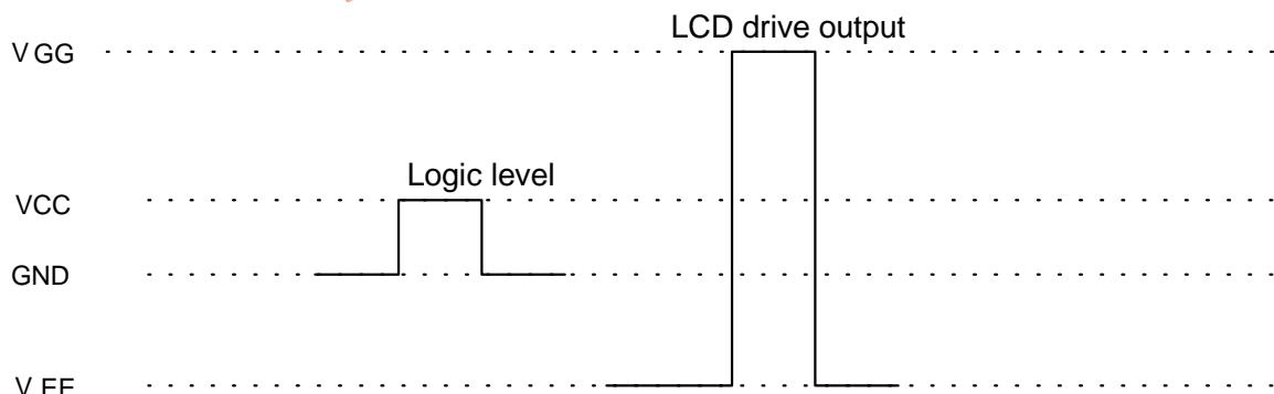
Note: For the input signals: CLK, XON, OE, U\_D, STVD & STVU, MODE, "High" level=VCC, "Low" level=GND
