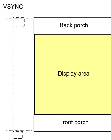
**Figure 5-7** Front porch and back porch function diagram
