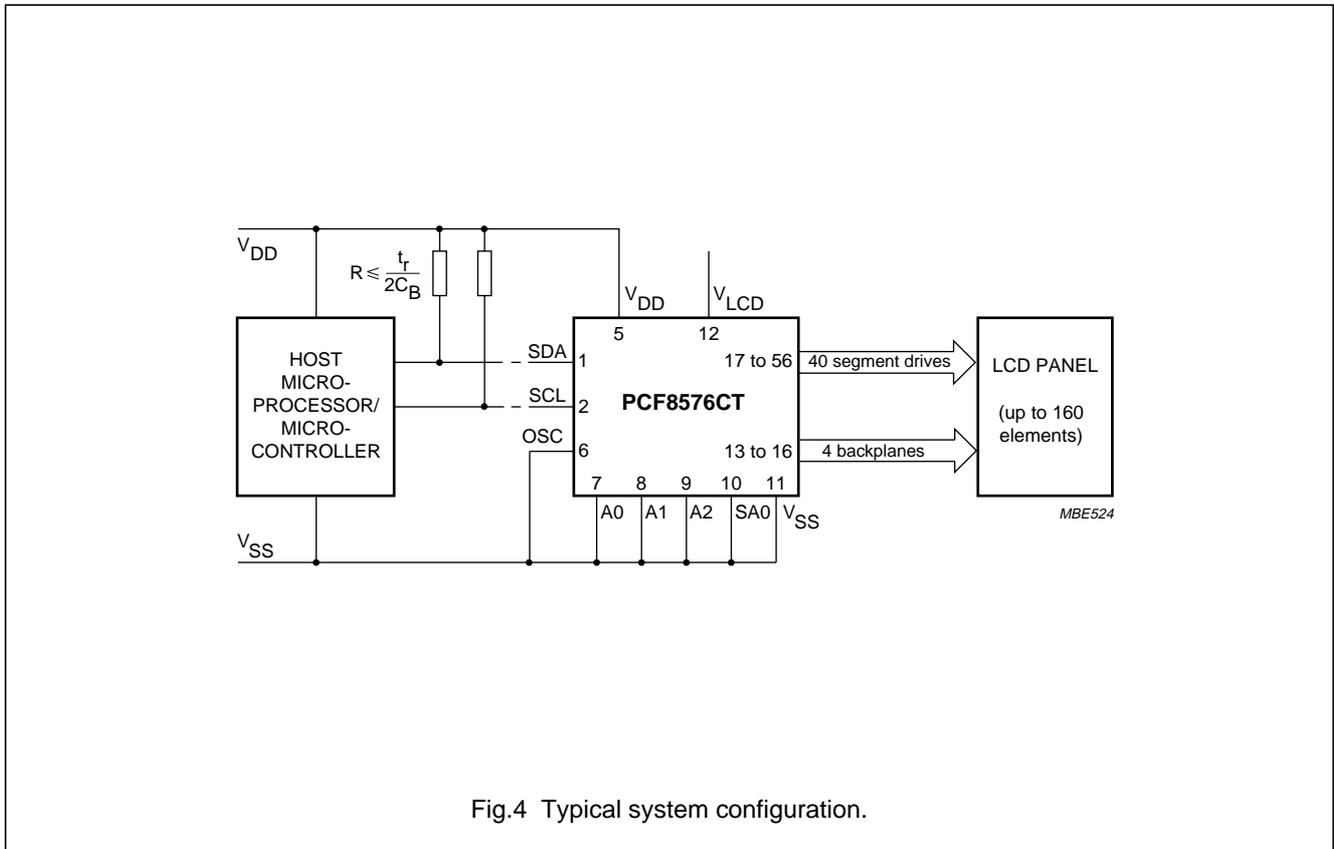
Fig.4 Typical system configuration.
