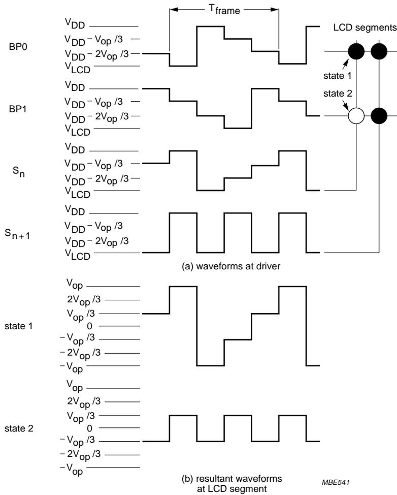
$$V_{state1}(t) = V_{S_n}(t) - V_{BP0}(t)$$
