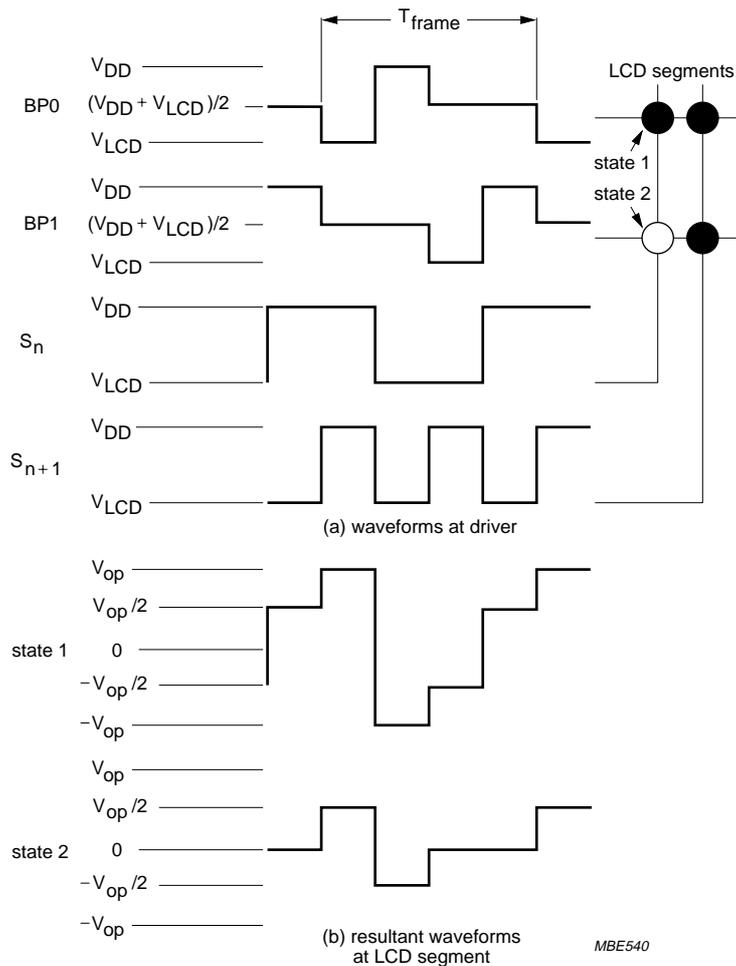
$$V_{state1}(t) = V_{S_n}(t) - V_{BP0}(t)$$
