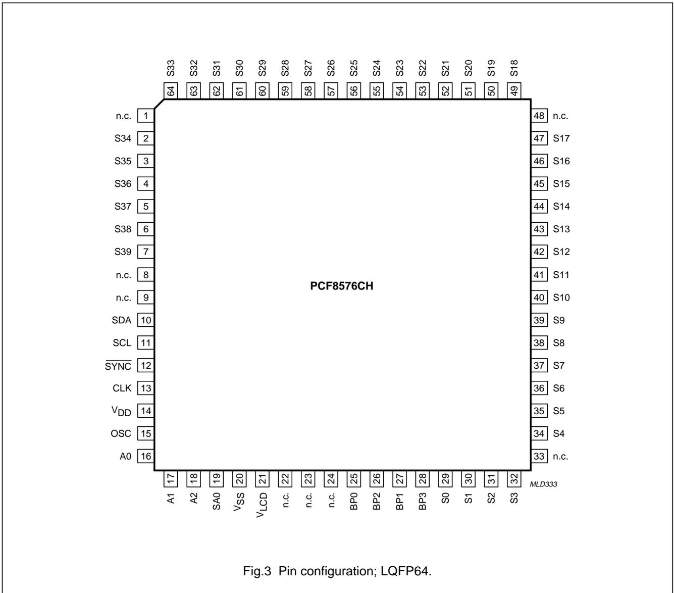
Fig.3 Pin configuration; LQFP64.
