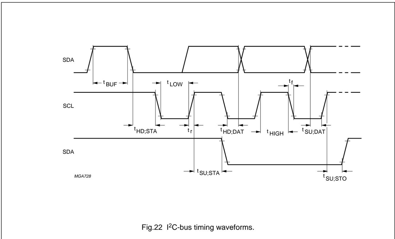
Fig.22 I<sup>2</sup>C-bus timing waveforms.
