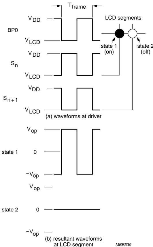
$$V_{state1}(t) = V_{S_n}(t) - V_{BP0}(t)$$
