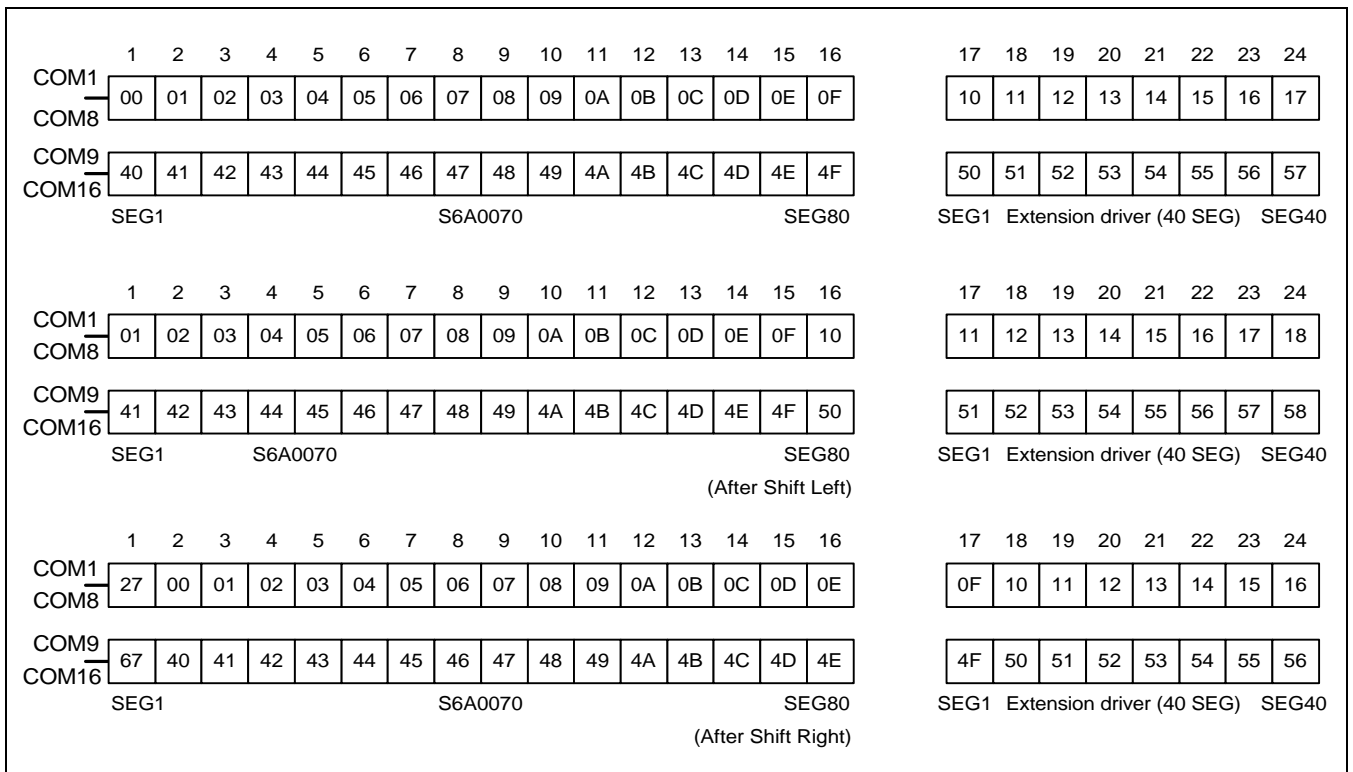
Figure 3. 2-line x 24ch. Display with 40 SEG. Extension Driver
