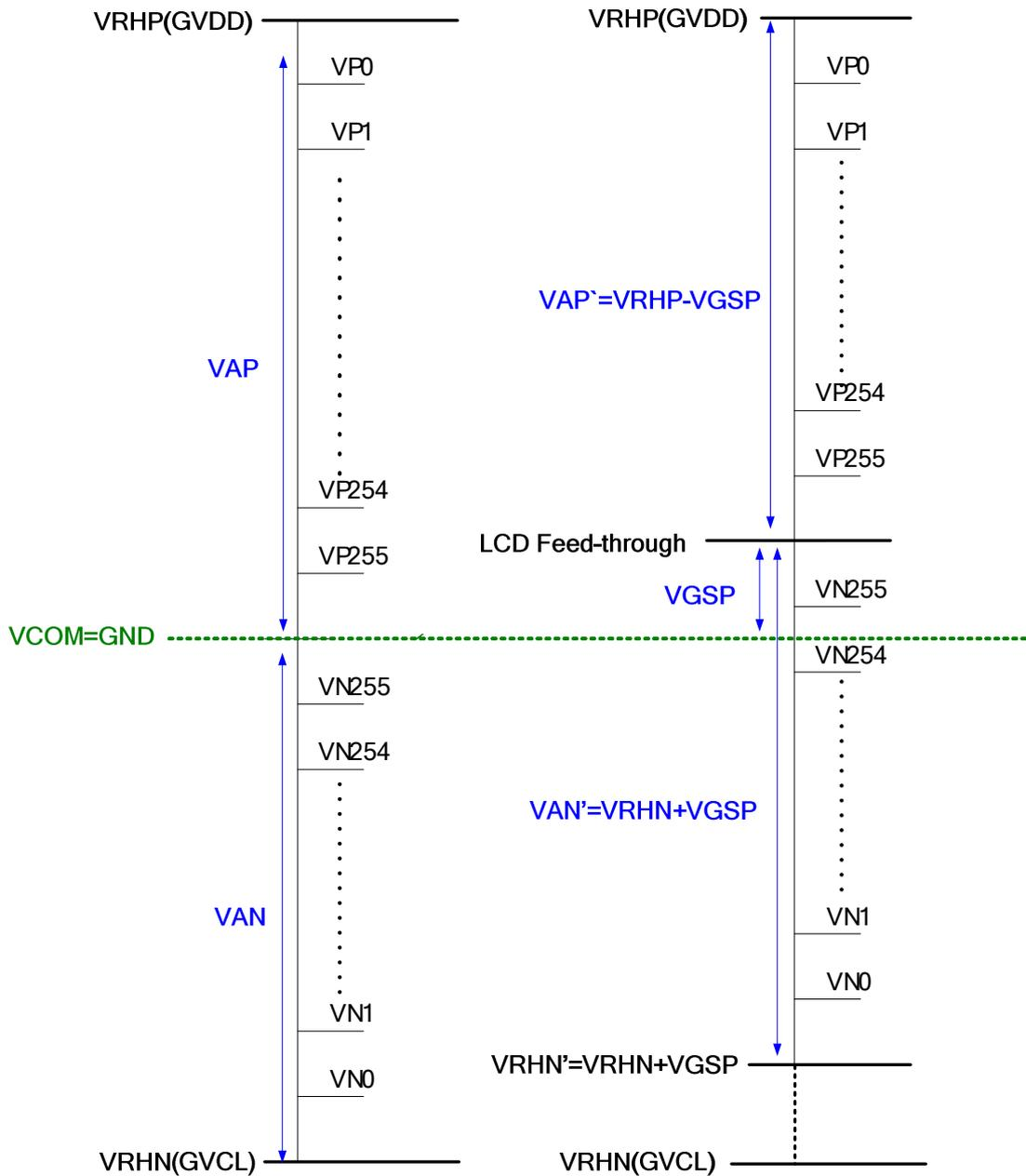
Note:  $VAP' = VRHP - VGSP$  and  $VAN' = VRHN + VGSP$  is LC voltage. Applied voltage between LC is 5.46~ 4.46V, and the difference depends on panel feed-through voltage (panel feed-through voltage estimation is 0.5~ 1.5V).
