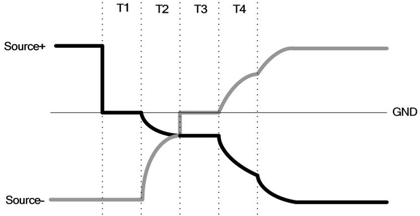
Source equalizing T4 time adjustment
