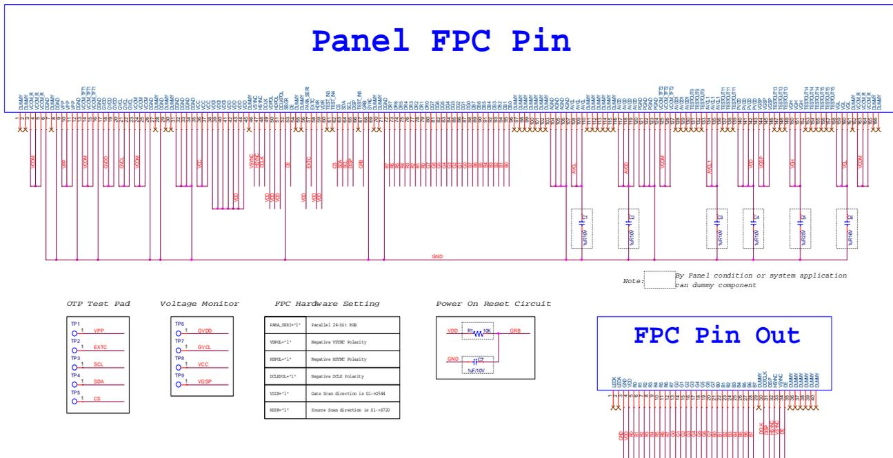
13.4.6 Serial RGB DE Mode Reference Circuit
