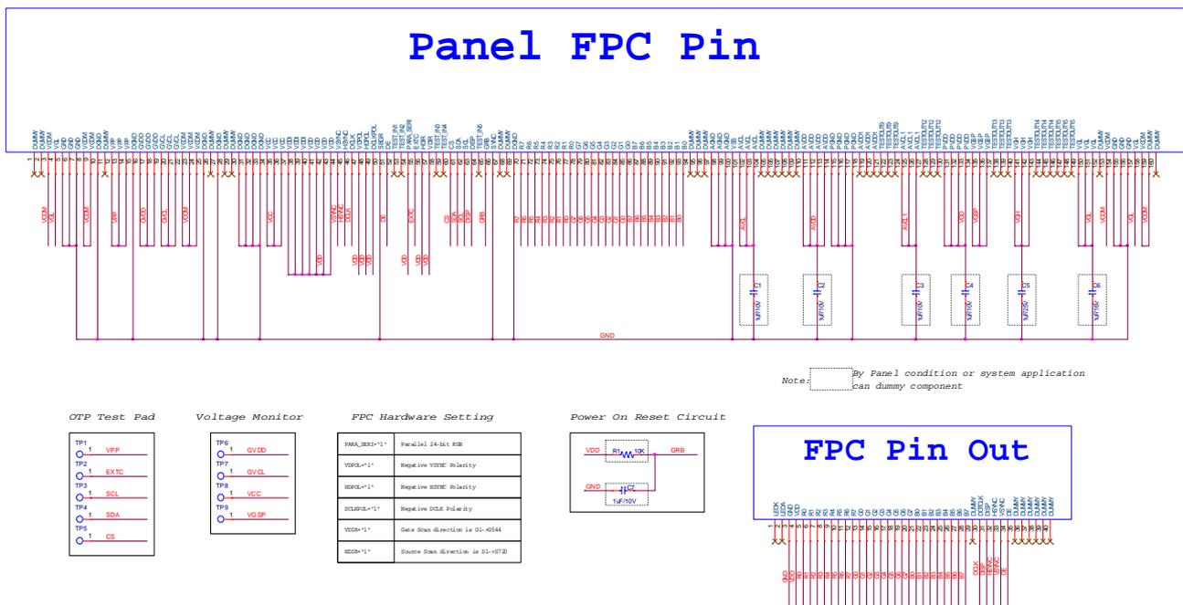
13.3.4 Serial RGB SYNC-DE Mode Reference Circuit
