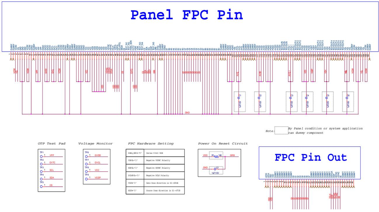
13.3.5 Serial RGB SYNC Mode Reference Circuit
