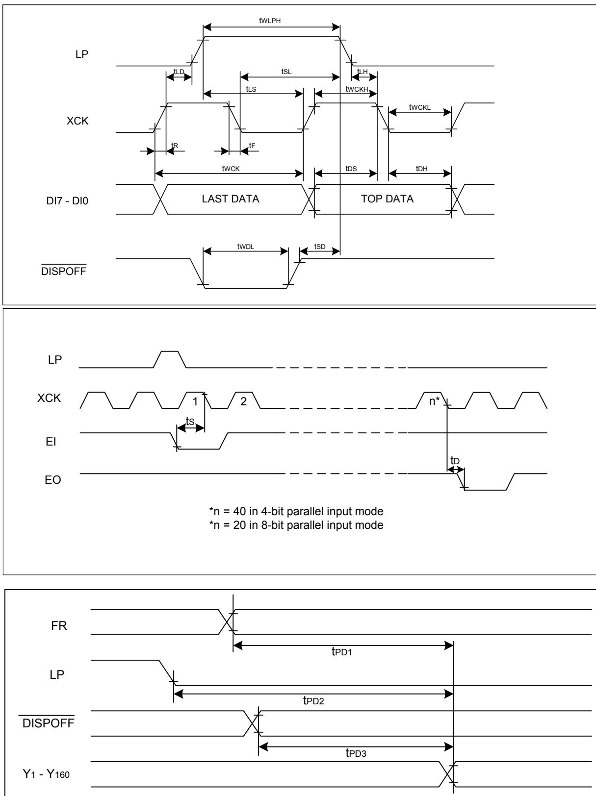
Fig. 8 Timing Characteristics (3)
