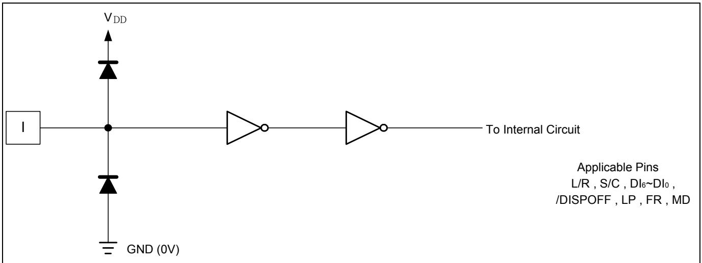
Figure 1 Input Circuit (1)
