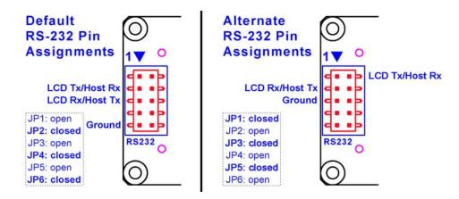
If there is a matching 0.1" center, 10-pin RS-232 connector on your system's motherboard, then in most cases a simple straight-through ribbon cable (such as CW Industries <u>C3AAG-1018G-ND</u>) can be used to connect from the CFA-633 to the motherboard's header. The pin order of your motherboard's header will determine if the CFA-633's pin assignments need to be "Default" or "Alternate".
