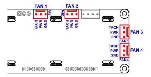
The average power delivered to each fan may be set to any level between 0% and 100%. The power setting controls the PWM duty cycle of a high-performance open-drain FET connected between the system ground and the GND pin of each fan connector. The PWM frequency is nominally 18Hz.
