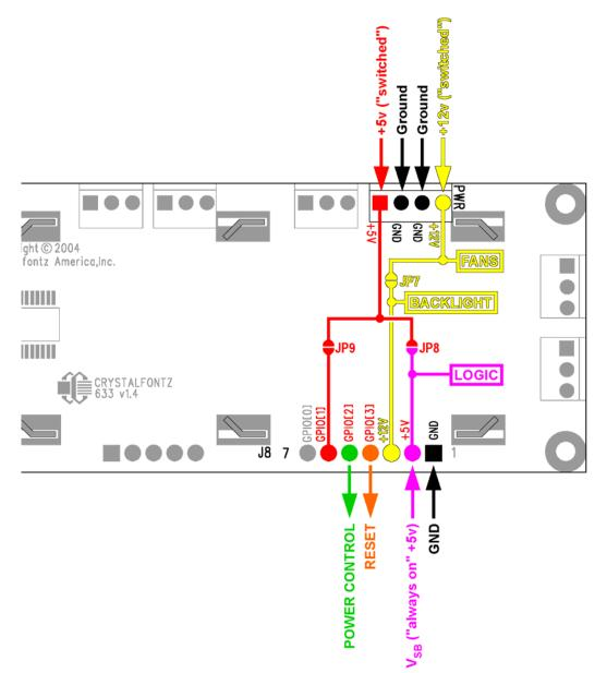
Once configured by the host software (<u>see command 28, Set ATX Power Switch</u> <u>Functionality</u>), the following functions may be individually enabled:
