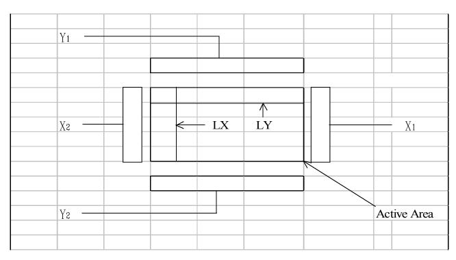
Voltage ( DC 5V) is applied to X1 or Y1 and GND to X2 or Y2 By using stylus to cross direct line for every 5 mm step within active area to detect the voltage at Y1 or X1
