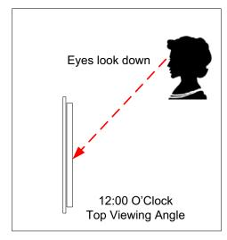
Figure 10. Definition of 6:00 O'Clock and 12:00 O'Clock Viewing Angles
