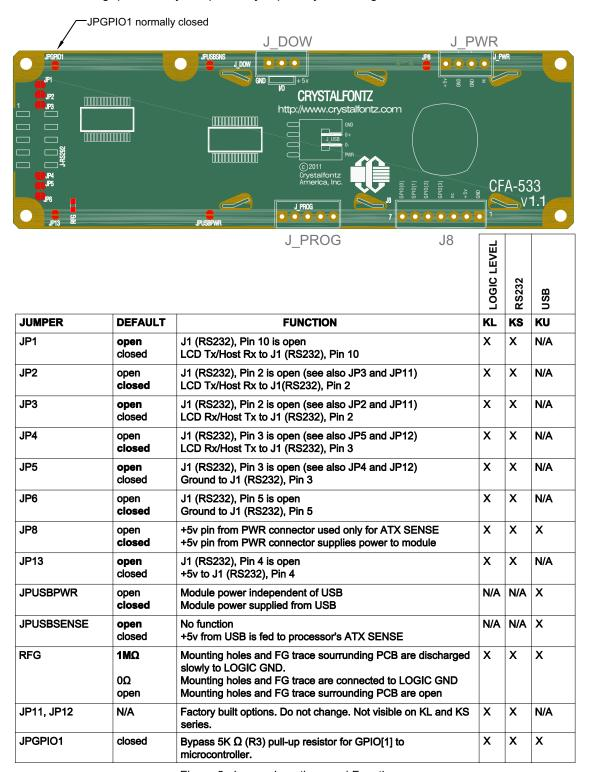
Figure 2. Jumper Locations and Functions
