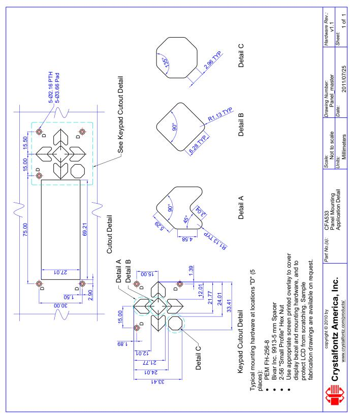
Figure 4. Panel Mounting Application Cutout Drawing
