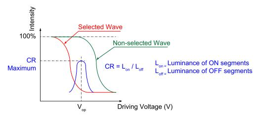
Figure 7. Definition of Operation Voltage (V<sub>OP</sub>) (Positive)
