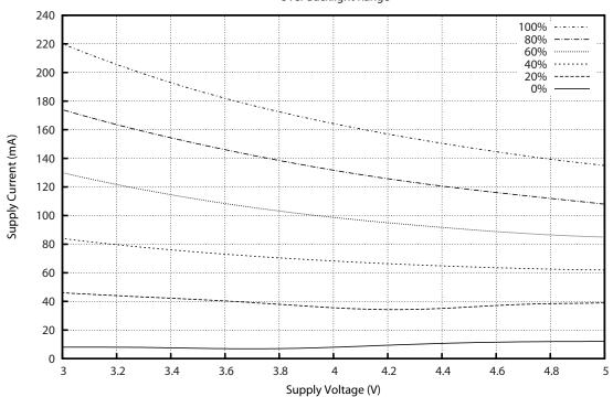
Figure 6. CFA533-YYH-KL Current Usage (same as CFA533-YYH-KS)
