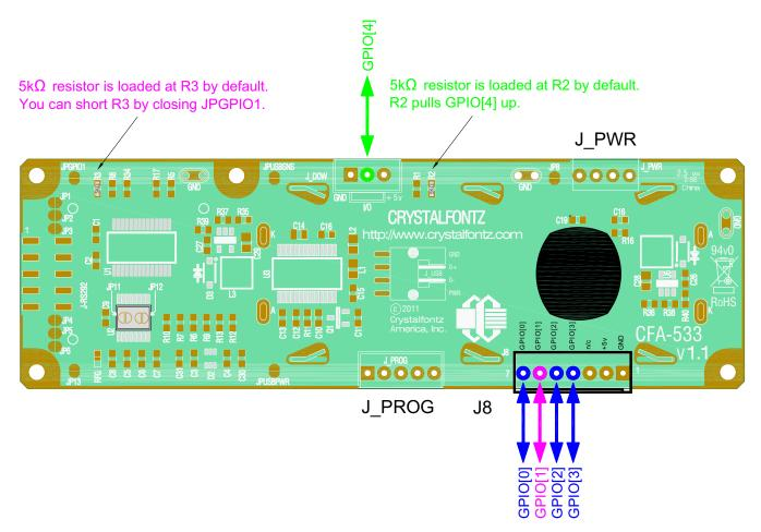
Figure 18. Location of GPIO Connections, Resistors, and J DOW
