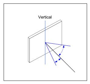
Figure 9. Definition of Horizontal and Vertical Viewing Angles (CR>2)
