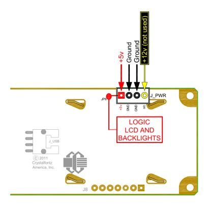
Figure 11. Standard (+5v) Connection through J\_PWR
