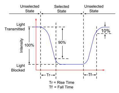
Figure 8. Definition of Response Time (Tr, Tf) (Positive)
