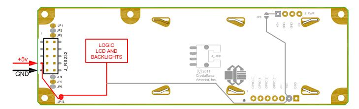
Figure 13. CFA533-YYH-KL Standard (+5v) Connection through J\_RS232 Connector
