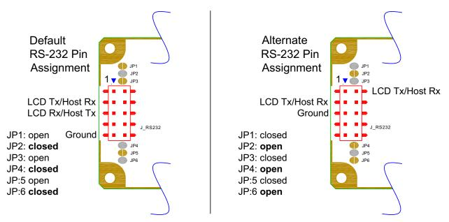
Figure 17. J\_RS232 Default and Alternate Pin Assignments
