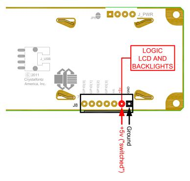
Figure 12. Standard (+5v) Connection through J8
