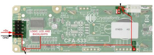
Remove RJP8 resistor to open JP8 when powering from the J\_RS232 Connector.
