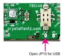
JP10 on the CFA735-xxx-KR is closed by factory default. If you are going to use USB interface while supplying power through H1, you must **open JP10** to prevent back-powering the USB.
