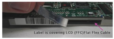
Bent FFC (Flat Flex Cable) is under the label.
