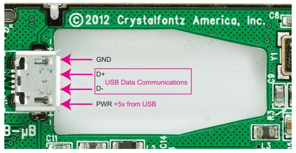
Figure 13. USB Connection Detail
