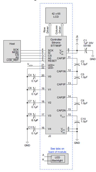
You must provide and connect capacitors C1 to C11 in order for the Sitronix ST7565 controller to generate the supply voltages for the LCD.
