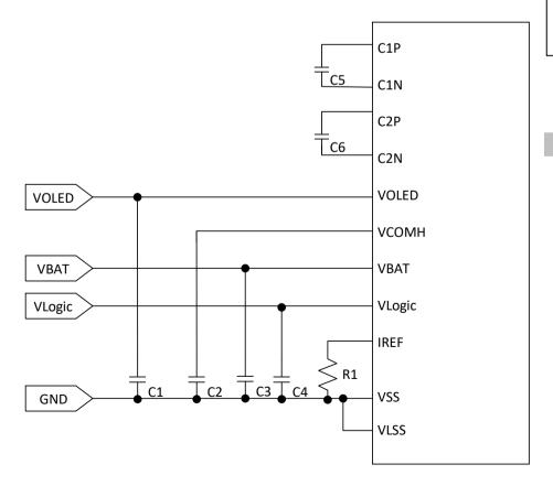
C1, C2:  $2.2\mu\text{F}$ C3, C4:  $1.0\mu\text{F}$ C5, C6:  $1.0\mu\text{F}/10\text{V}$ R1=(V<sub>IREF</sub>-V<sub>SS</sub>)/I<sub>REF</sub>  $\approx 300\text{k}\Omega$
