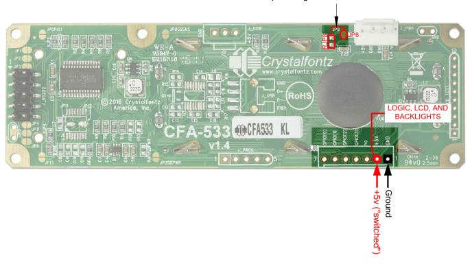
Figure 10. Standard Power Supply Connection Through J8
