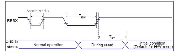
VDDI=1.65 to 3.3V, VDD=2.4 to 3.3V, AGND=DGND=0V, Ta=-30 ~ 70 °C
