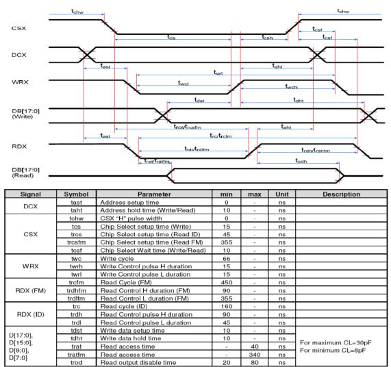
Note: Ta = -30 to 70 ℃, IOVCC=1.65V to 2.8V, VCI=2.6V to 3.3V, GND=0V
