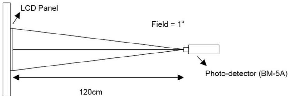
Figure 7. Definition of Optical Measurement Set-up
