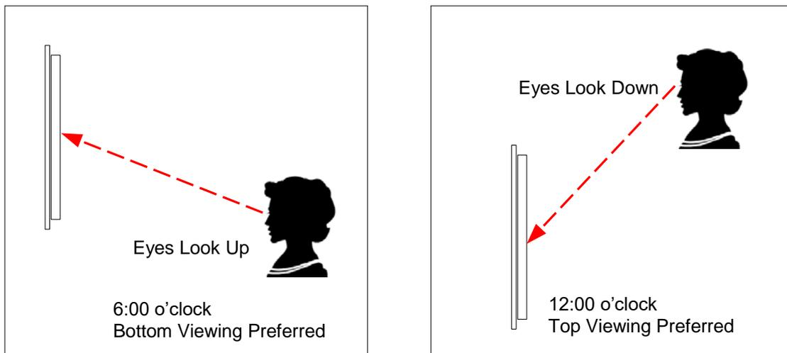
Figure 5. Definition of 6:00 o'clock and 12:00 o'clock Viewing Angles
