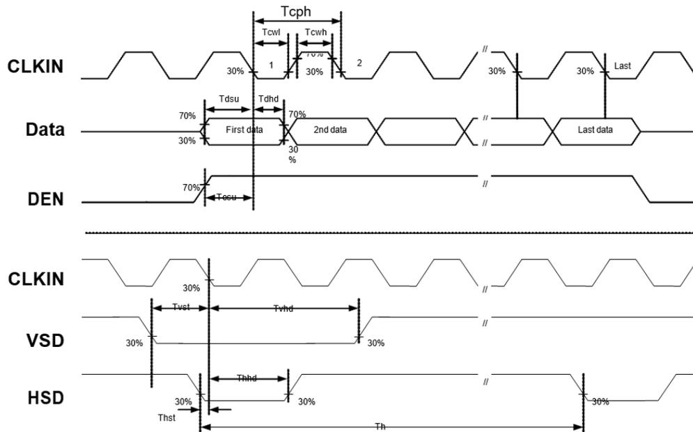
Figure 2. Clock Timing Sample
