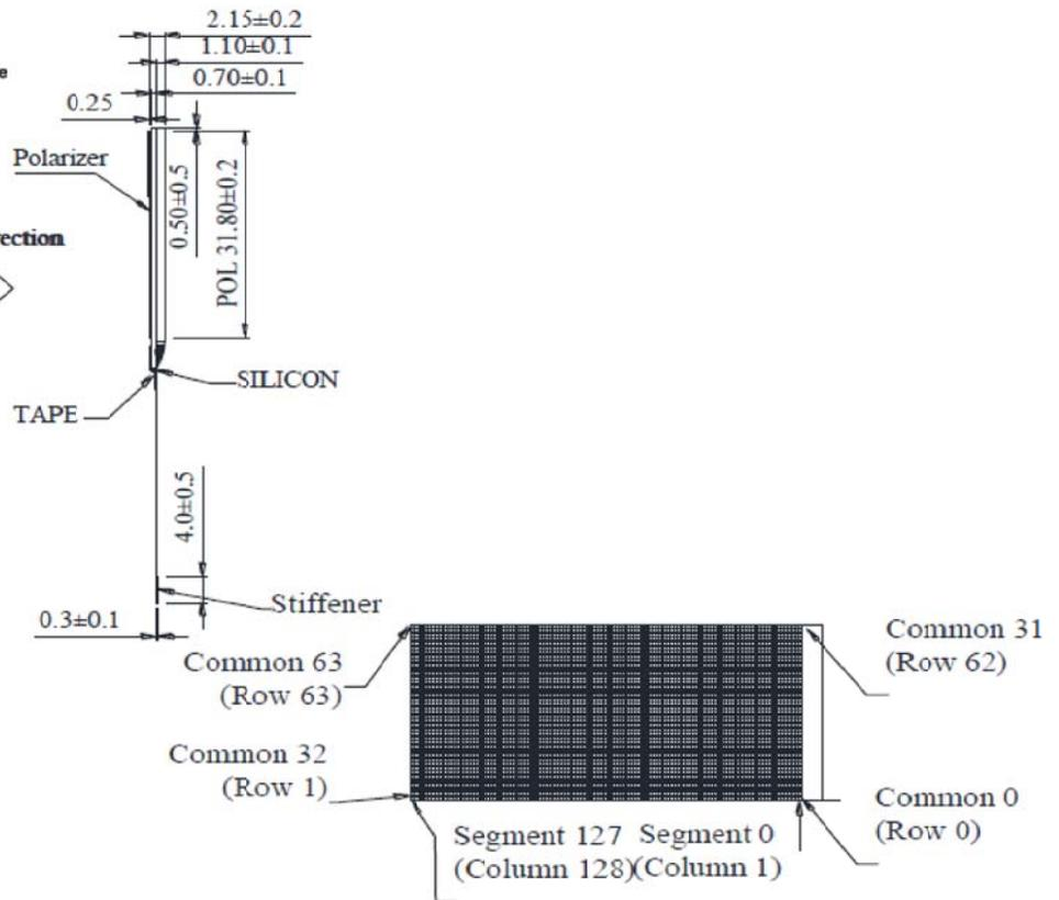
Tolerance is  $\pm 0.3\text{mm}$  unless specified.
