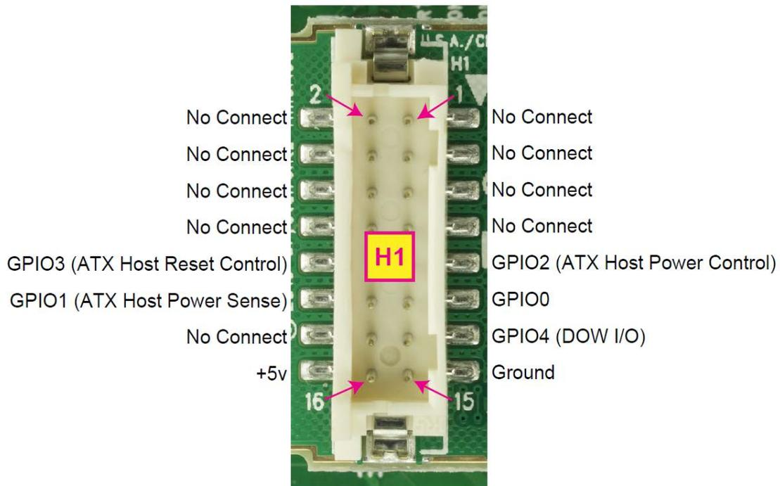
Figure 7. Pin Assignments on CFA635-xxx-KU H1 Connector
