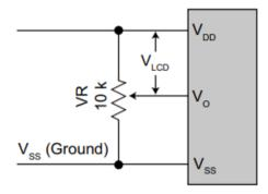
We recommend allowing field adjustment of  $V_O$  for all designs. The optimal value for  $V_O$  will change with temperature, variations in  $V_{DD}$ , and viewing angle.  $V_O$  will also vary module-to-module and batch-to-batch due to normal manufacturing variations.
