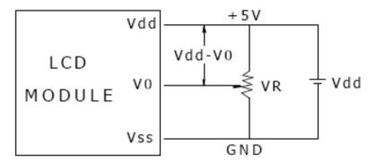
Vdd-V0: LCD Driving Voltage
