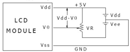
Vdd-V0: LCD Driving Voltage
