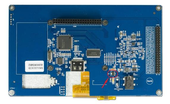
10.1" displays CFAM1280800A0-101C, -101N, and -101R – Remove U6
