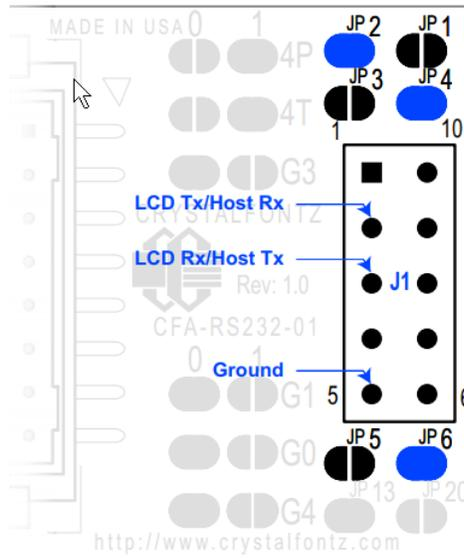
Figure 16. CFA-RS232 J1 Connector Default RS232 Pin Assignments
