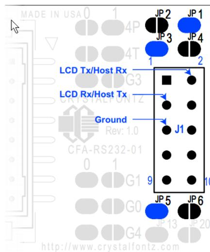
Figure 17. CFA-RS232 J1 Connector Alternate RS232 Pin Assignments
