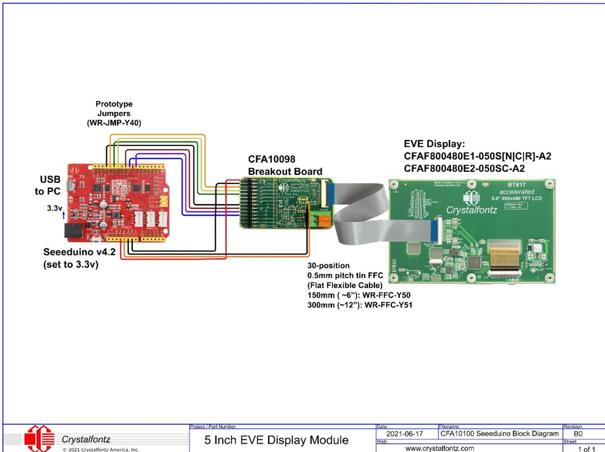
If your kit ships with the flex cable disconnected, take note of the orientation of the flat-flex-cable, and use of the locking clip in the following photos.
