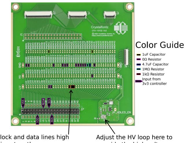
Pull I2C clock and data lines high Tie data lines together Adjust the HV loop here to provide the high voltage (VCC 12-14v)
