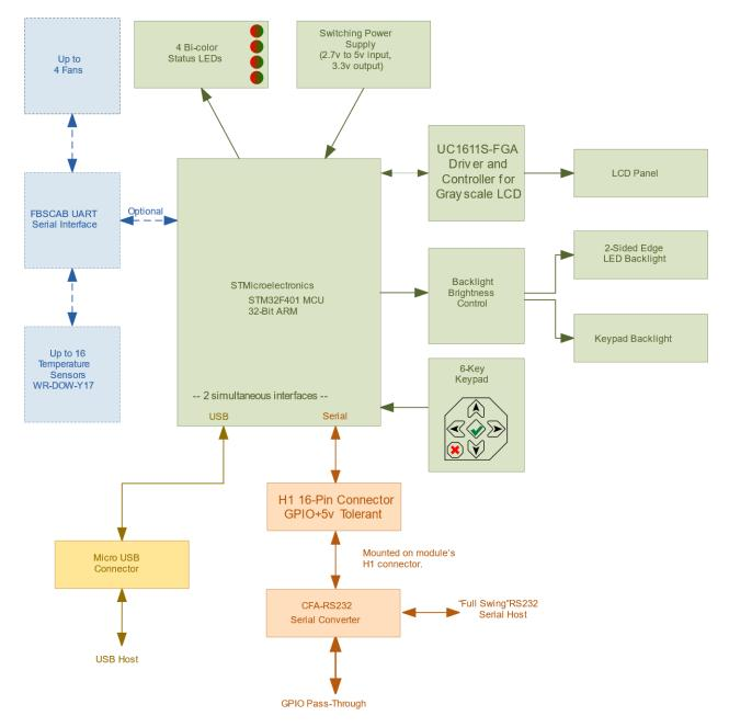
Figure 4. System Block Diagram – CFA735-xxx-KT
