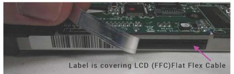
To avoid damaging the FFC, handle the module with care and avoid any pressure along the sticker.
