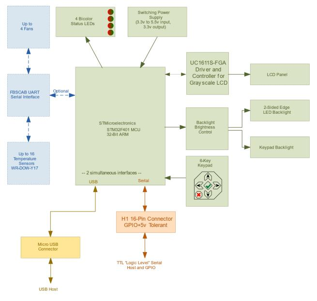
Figure 3. System Block Diagram – CFA735-xxx-KR
