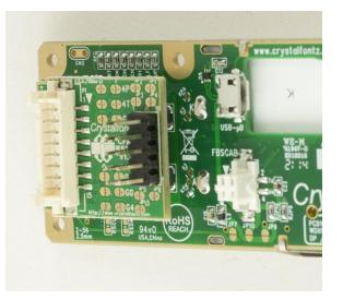
Figure 12. Angled View of CFA-RS232 Level Translator Mounted on CFA735-xxx-KR
