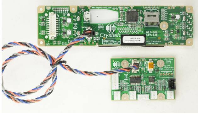
Figure 19. CFA735 Connected to Optional FBSCAB Using WR-EXT-Y37 Cable
