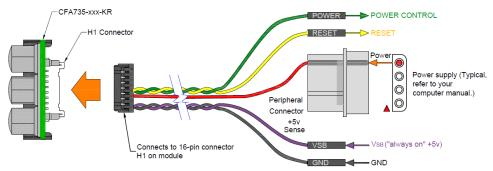
Figure 9. CFA735-xxx-KR ATX Connection to H1 with WR-PWR-Y25 or WR-PWR-Y38 Cable
