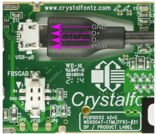
Figure 7. Connecting 5v Power Through USB
