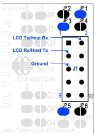
Figure 17. CFA-RS232 J1 Connector Alternate RS232 Pin Assignments
