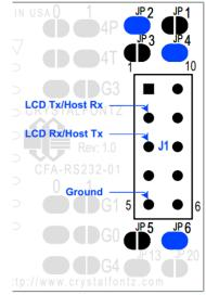
Figure 16. CFA-RS232 J1 Connector Default RS232 Pin Assignments
