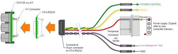
Figure 10. CFA735-xxx-KT ATX Connection to H1 with WR-PWR-Y25 or WR-PWR-Y38 Cable
