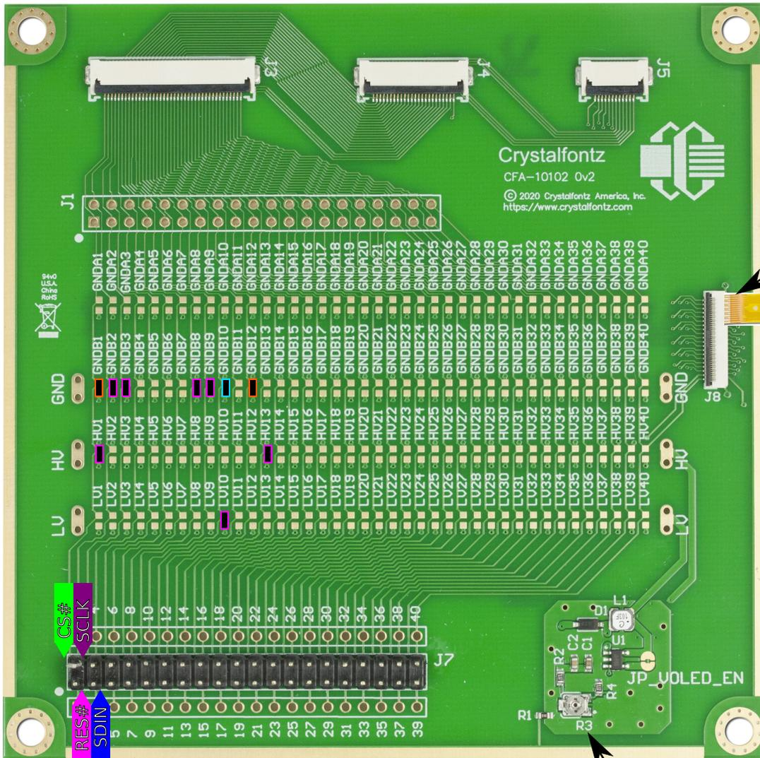
Carefully align the ZIF tail to the top of the ZIF connector and close the connector.
