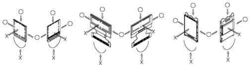
Do not apply stress to the LSI chips and the surrounding molded sections.
