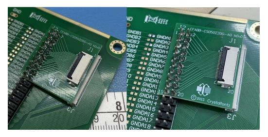
There are two limitations to using the CFA10102 in this manner. The first is that the adapter board can only support a maximum of 40 pins. The second is that, in most cases, J3 cannot be used after the board has been soldered.
